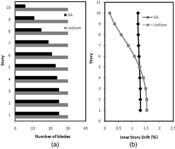
Figure 4. Optimized device configuration for inter-story drift
