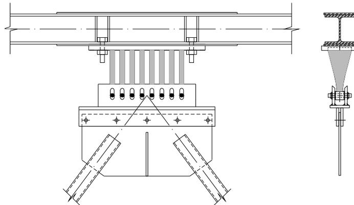
**Figure 1.** Triangular-plate Added Damping and Stiffness (TADAS) and typical configuration
