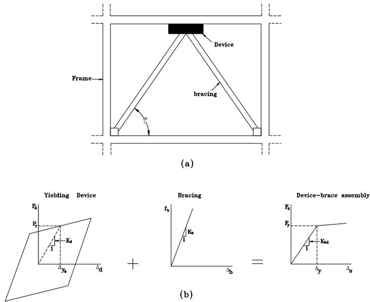
**Figure 3.** Yielding metallic damper, (a) typical configuration, (b) yielding metallic device, bracing and yielding element parameters
