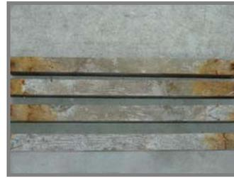
**Figure 2.5.** The appearance of RC members after corrosion
