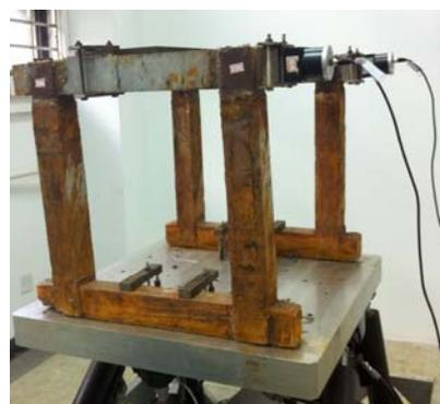
Figure 3.3. Experimental instruments for dynamic test of frame
