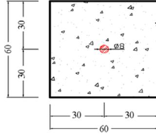
**Figure 2.1.** Reinforcement arrangement of beams
