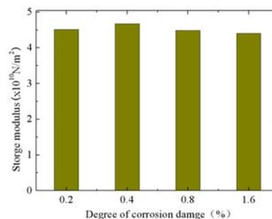
**Figure 2.7.** Influence of steel-bar corrosion on storage modulus
