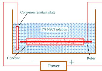
**Figure 2.4.** Electro-chemical accelerated corrosion device
