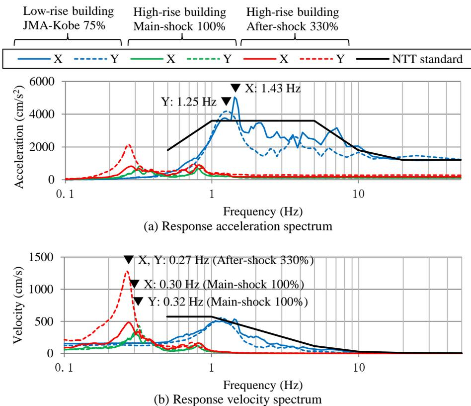
**Figure 6.** Comparison of the response spectrum (P1FL h=3%)
