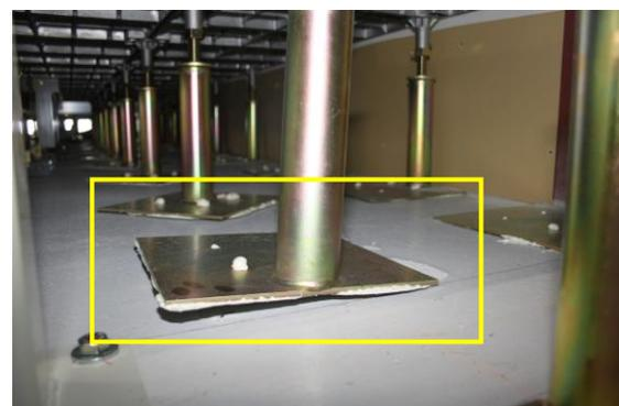
(d) Flaking of column bases between paintwork and floor slab (JMA-Kobe 75%)
