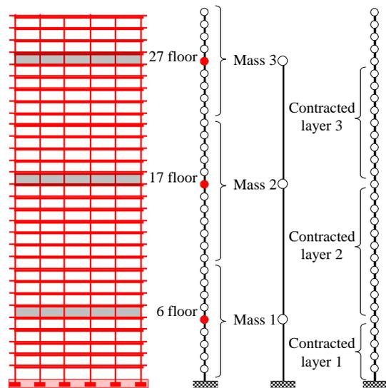
Figure 2. Remodeled and scaled down method of high-rise building
