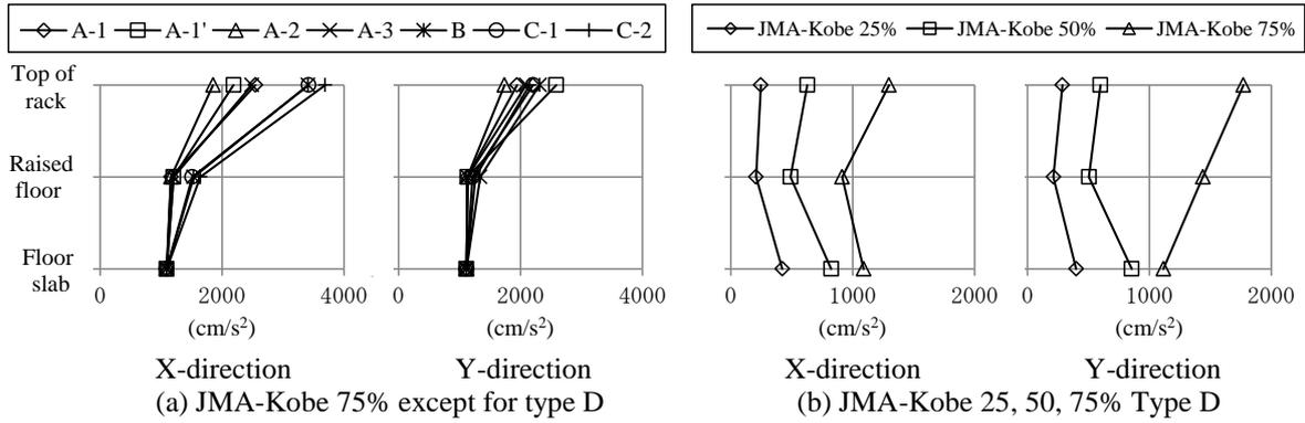
**Figure 9.** Maximum response acceleration in the low-rise building
