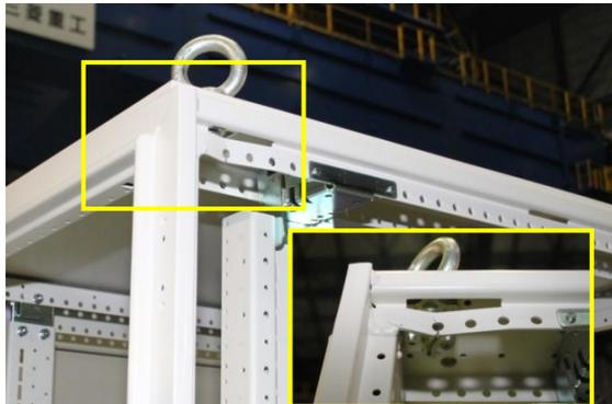
(c) Crack of welded part of rack (JMA-Kobe 75%)
