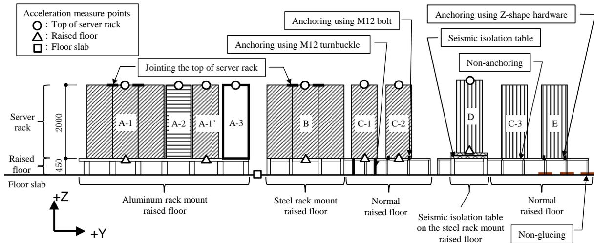
Figure 5. Elevation of the telecommunications equipment
