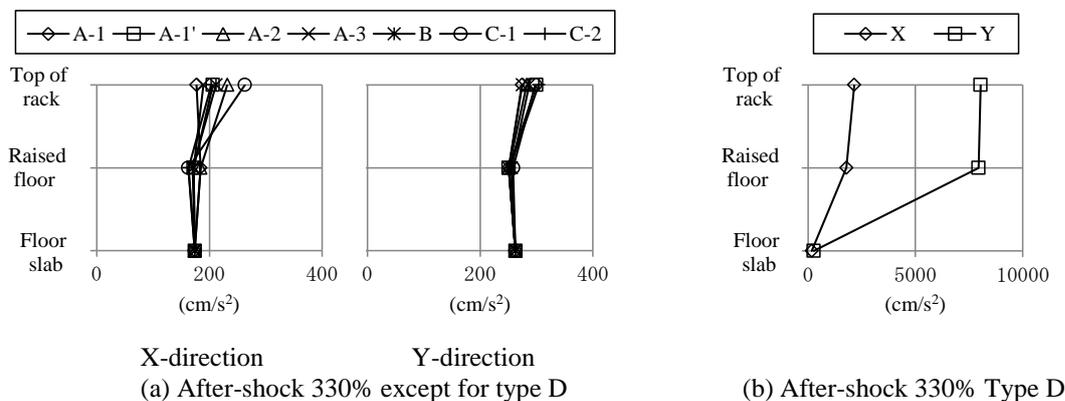
Figure 8. Maximum response acceleration in the high-rise building
