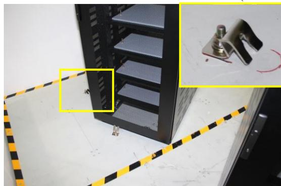
(e) Damage of Z-shape hardware and move of rack (JMA-Kobe 75%)
