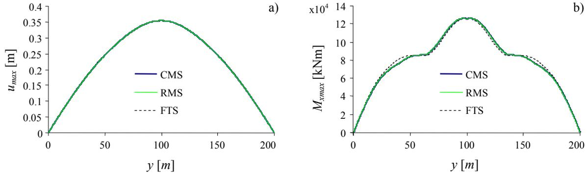
**Figure 4.** Transverse displacements and bending moments along the deck according to the exact and the simplified analysis techniques.
