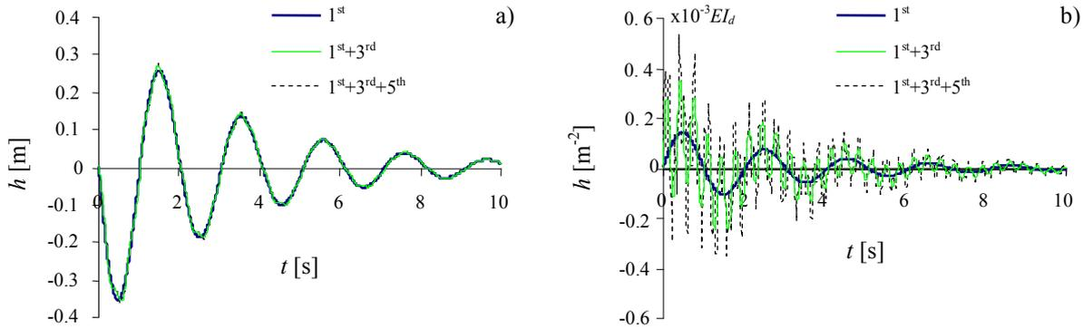
**Figure 2.** Response to impulsive loading in terms of a) midspan transverse displacement and b) abutment reactions.
