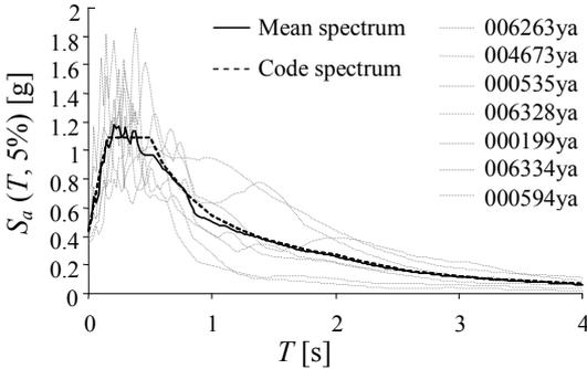
**Figure 3.** Input response spectrum and response spectra of natural records vs period  $T$ .
