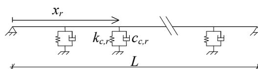
**Figure 1.** Analytical 2-dimensional model for PRSI bridges.
