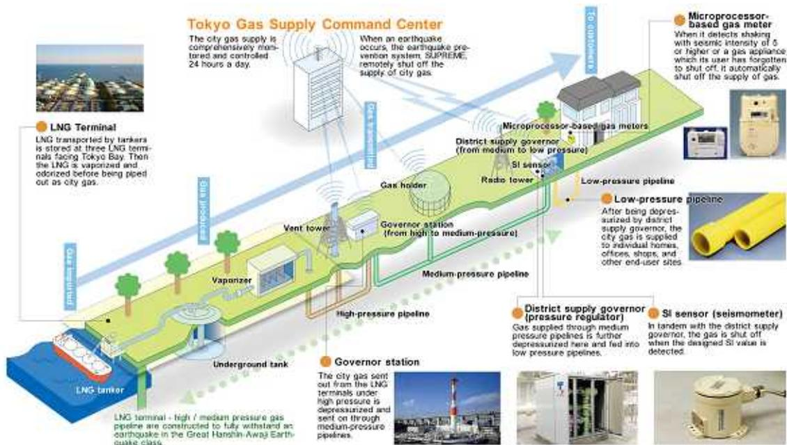
Figure 1. Outline of the City Gas Supply System and Earthquake Safety Measures
