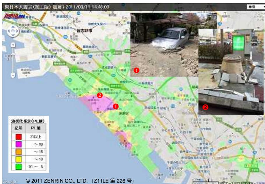
**Figure 4.** Estimation of Risk of Liquefaction by SUPREME and Actual Liquefaction Damage
