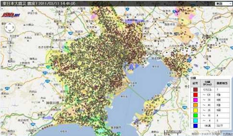
Figure 3. SI value observed by SI Sensors and Interpolated SI Values by 50m Meshes
