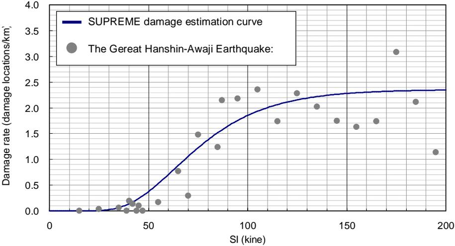
**Figure 2.** Damage Estimation Curve of SUPREME
