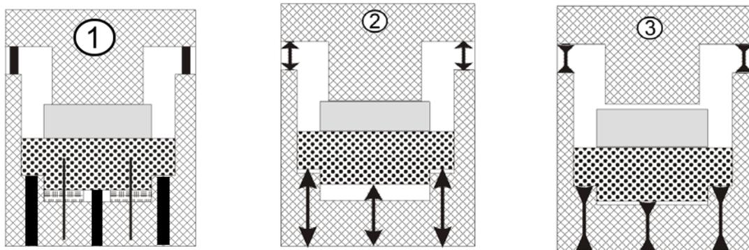
a) Insertion of the hydraulic presses b) Uplifting of the concrete block c) Lowering of the concrete block
