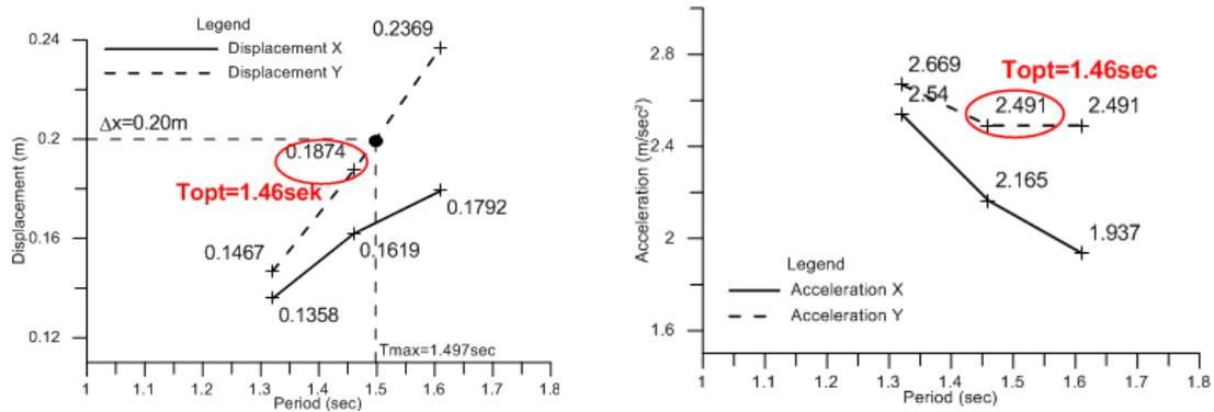
a) Shear deformation at the isolation level      b) Acceleration at the top of the structure
