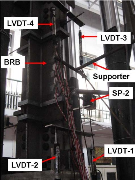
**Figure 4.1.** Photo of component test setup
