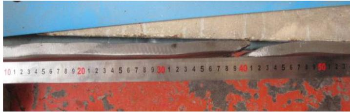
**Figure 4.6.** Multi-wave buckling of the core plate of BRB-2
