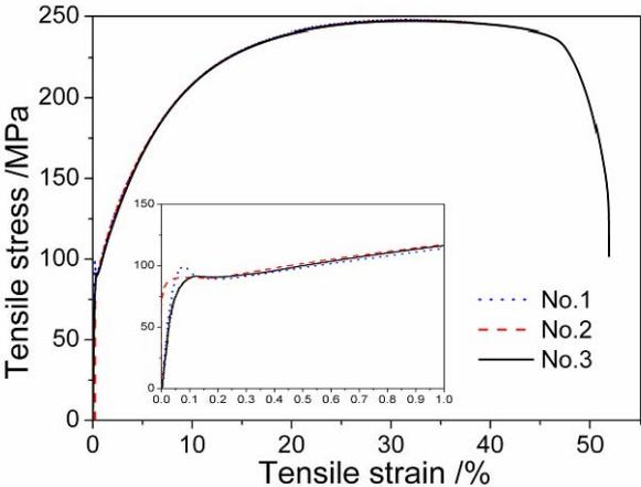
**Figure 2.1.** Relationships between tensile stress and tensile strain of three Q100 steel samples
