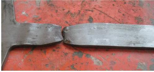
**Figure 4.3.** Failure mode of BRB-1
