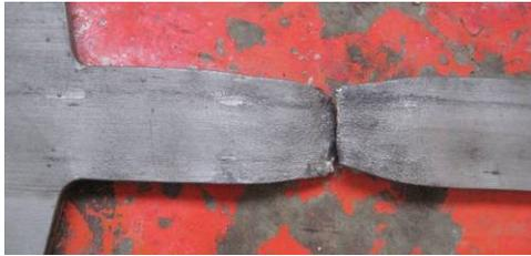
**Figure 4.5.** Failure mode of BRB-2
