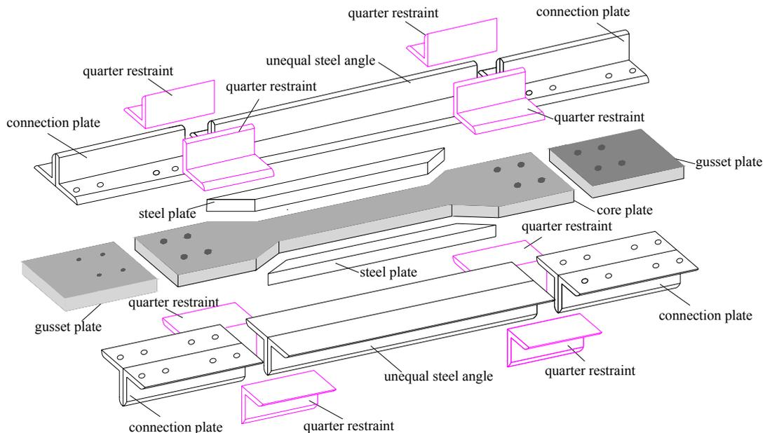
**Figure 3.1.** Configuration of BRB specimen
