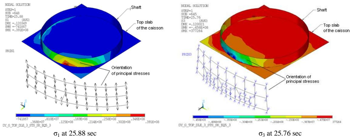
**Figure 10.** Zones with main stresses under seismic impact of DLE level at the shaft joint with the top slab of the caisson (Pa)
