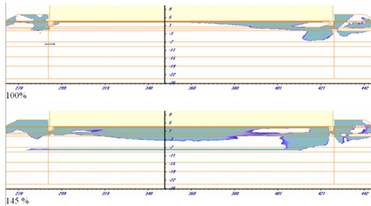
**Figure 4.** Plastic deformation zones under horizontal seismic loading
