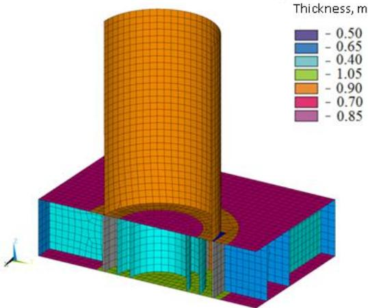
Figure 6. 3D fragment of the shaft model
