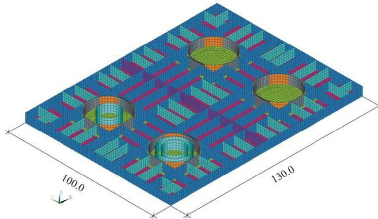
**Figure 7.** Caisson model section by a horizontal plane
