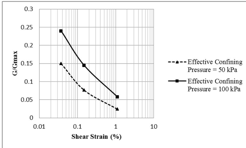
**Figure 6.1.** Influence of eff. confining press. on normalized shear modulus vs shear strain at 0.25% coir fiber
