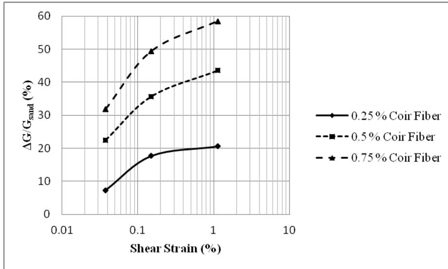
**Figure 5.5.** Percent increase in shear modulus with coir fiber content at different shear strains
