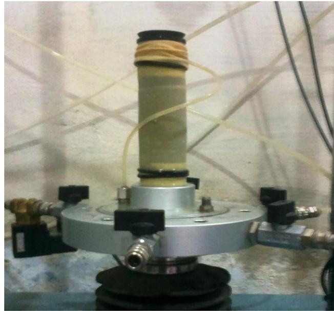
**Figure 3.1.** A sample ready for testing on cyclic triaxial
