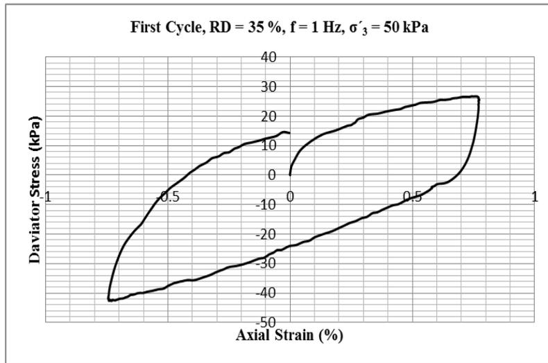
**Figure 5.1.** Deviator stress vs. axial strain at first cycle for sand with 0.25% coir fiber at 0.75% axial strain
