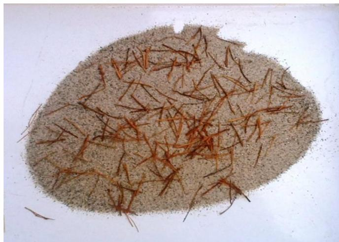
**Figure 2.2.** A typical sample of coir fibers used in the study
