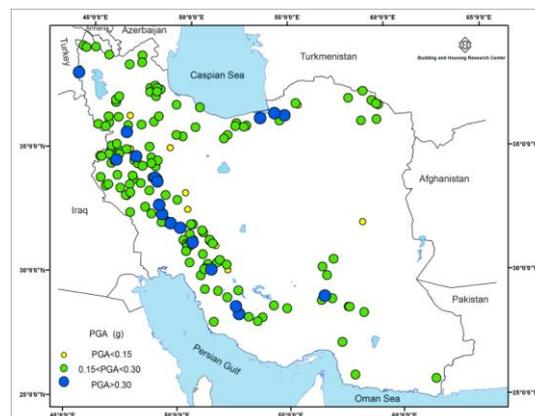
**Figure 5.** Estimated PGA's for the sites of important structures in Iran
