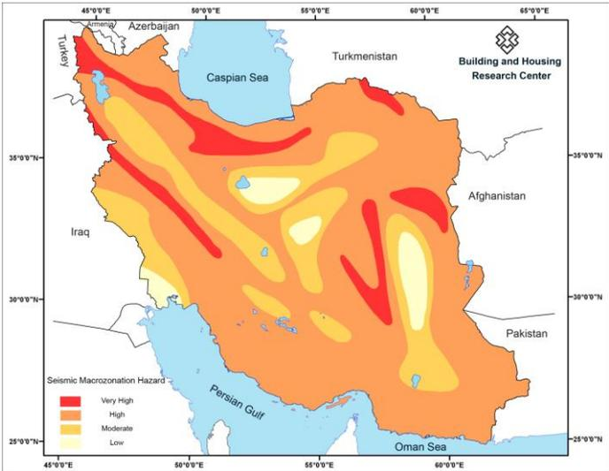
Figure 6. New seismic hazard zoning map of Iran
