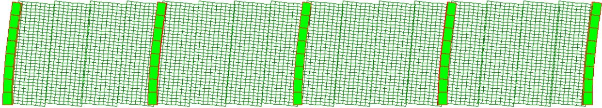
**Figure 2.** Disconnected vertical panels: deformation of the structure ( $d_{top}=73,0$  mm).
