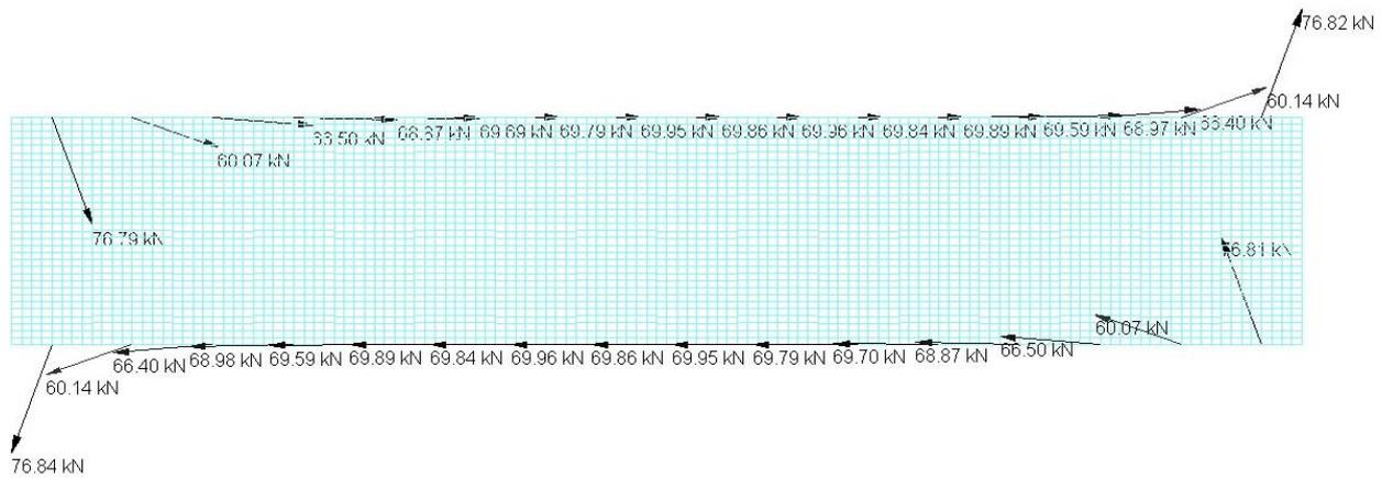
**Figure 3.** Rigid connections among vertical panels: reaction forces on the fastenings (kN).
