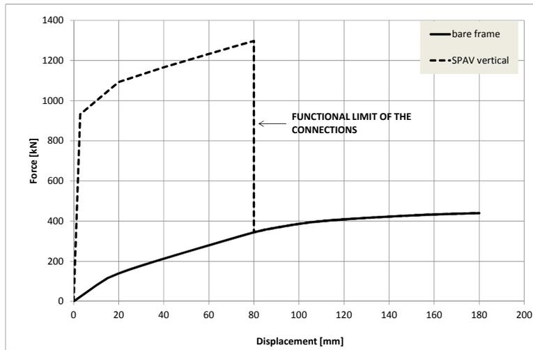
**Figure 6.** Pushover curve with SPAV connections for the structural system with vertical panels.
