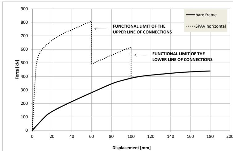
**Figure 13.** Pushover curve with SPAV connections for the structural system with horizontal panels.
