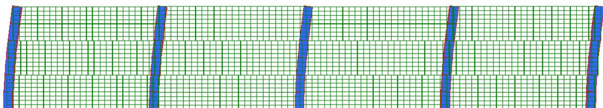
**Figure 11.** Disconnected horizontal panels: deformation of the structure ( $d_{top}=73,0$  mm).
