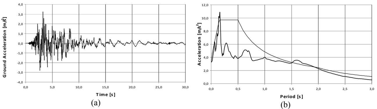
**Figure 7.** L'Aquila earthquake (AQK-WE): (a) accelerogram, and (b) response spectrum compared with the model of EC 8.
