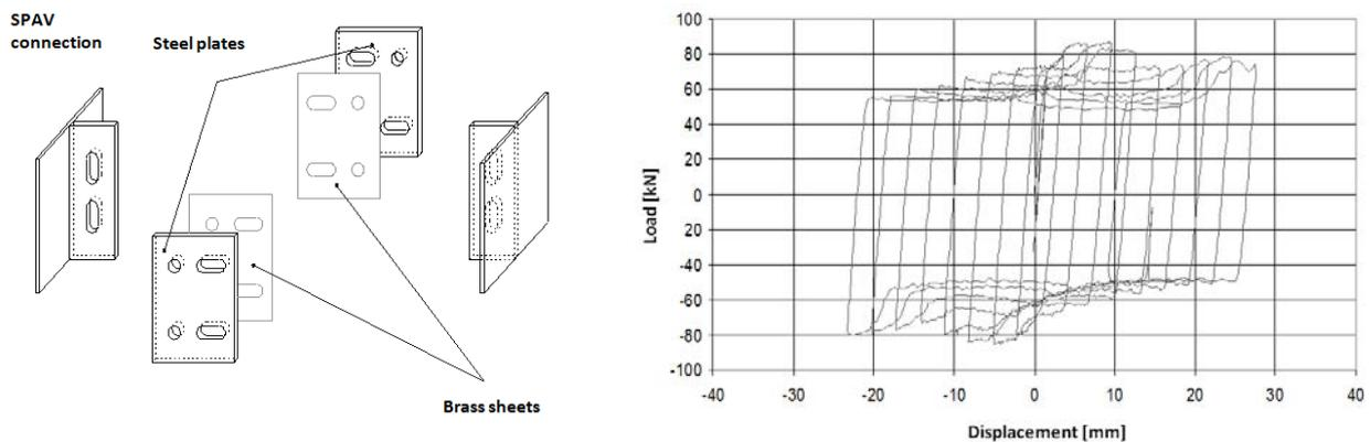
**Figure 5.** Components of SPAV connection and experimental load-displacement cycles.
