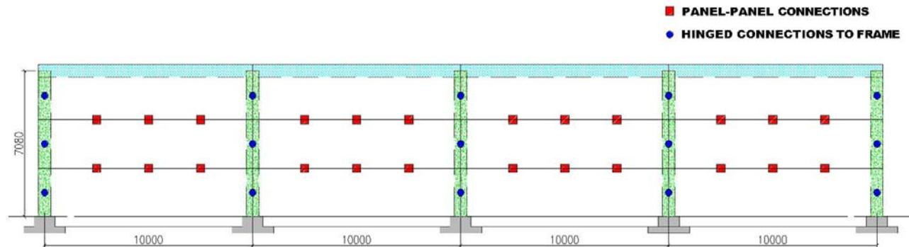
**Figure 10.** View of the cladding wall system with horizontal panels.
