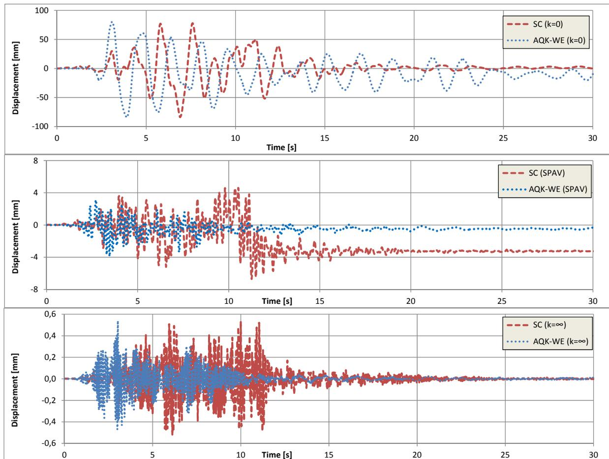
**Figure 9.** Displacement time histories under L'Aquila earthquake (AQR-WE) and the artificial accelerogram (SC).
