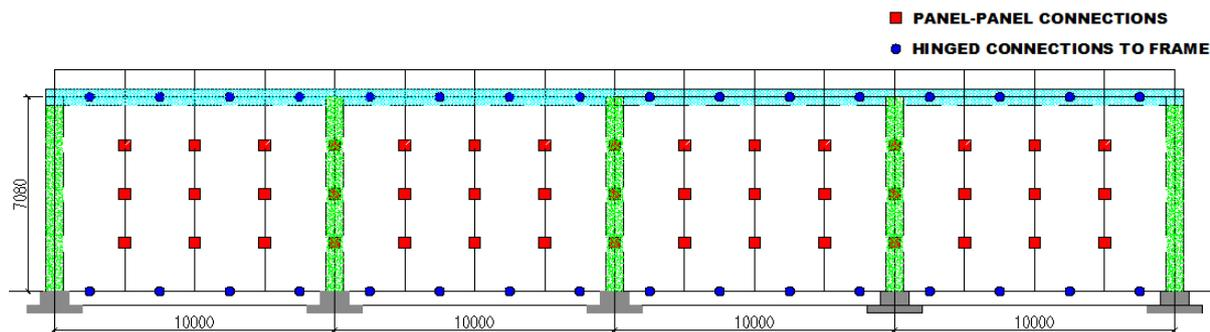
**Figure 1.** View of the cladding wall system with vertical panels.
