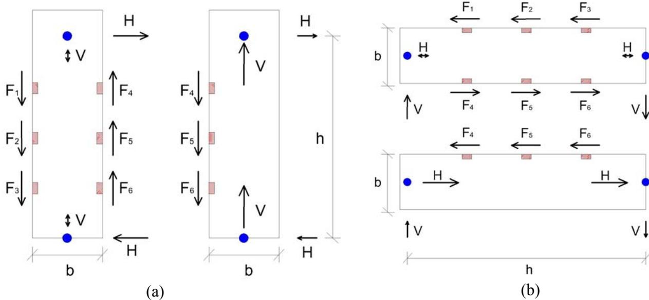
**Figure 15.** Equilibrium of (a) vertical and (b) horizontal cladding panels with connections.
