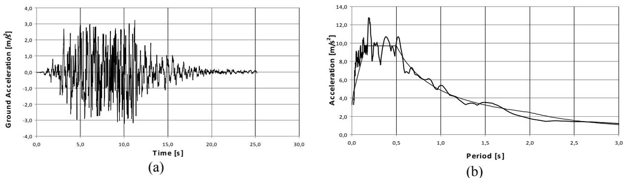
**Figure 8.** Artificial earthquake (SC): (a) accelerogram, and (b) response spectrum compared with the model of EC 8.
