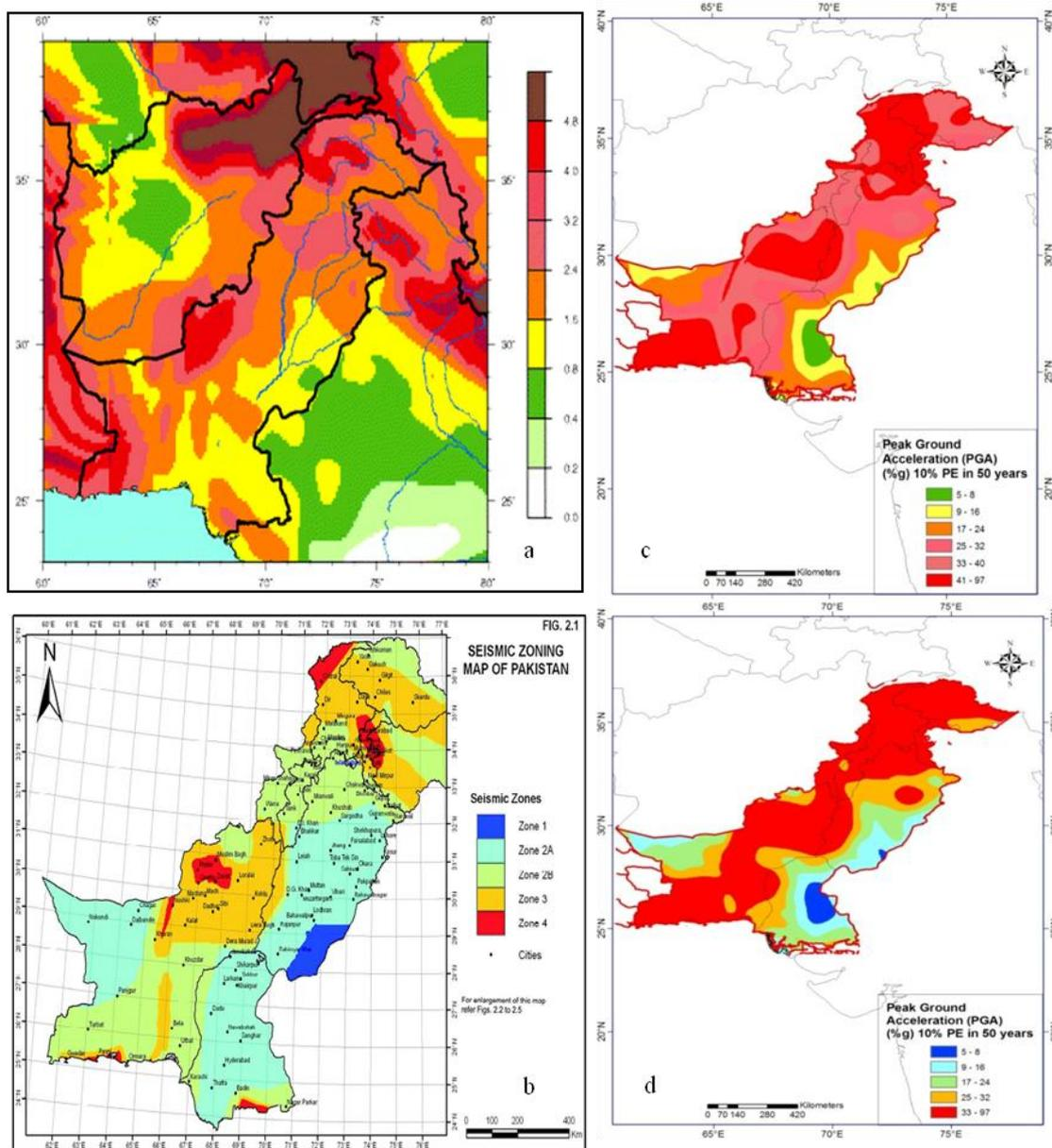
**Figure 8** Comparison of PGA maps with 10% PE in 50 years developed by (a) GSHAP 1999, (b) NESPAC 2007 , (c) and (d) This Study—2012
