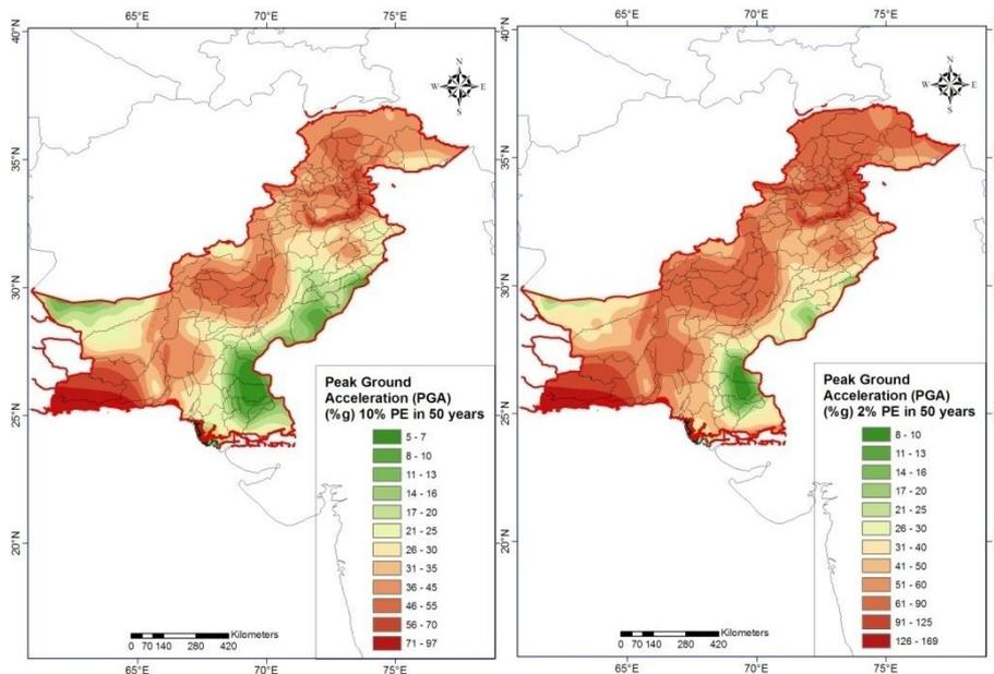
**Figure 7.** Map of peak ground acceleration (PGA) for 10% PE in 50 years and 2% PE in 50 years in Pakistan in standard gravity (% g)
