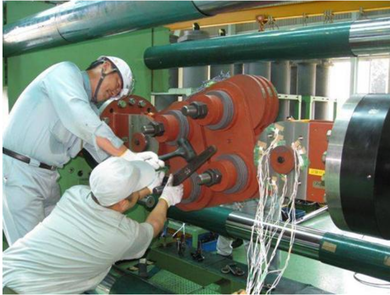
Figure 8. Test setup of 1500 kN damper at Kawakin Testing Facilities in Japan
