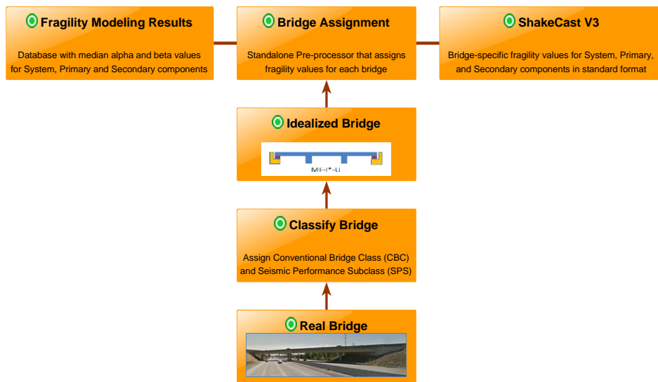
Figure 7. Converting g2F component-based fragility modelling to ShakeCast fragility curves
