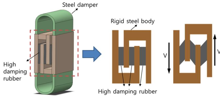
**Figure 2.** Shape of Hybrid Energy Dissipative Device
