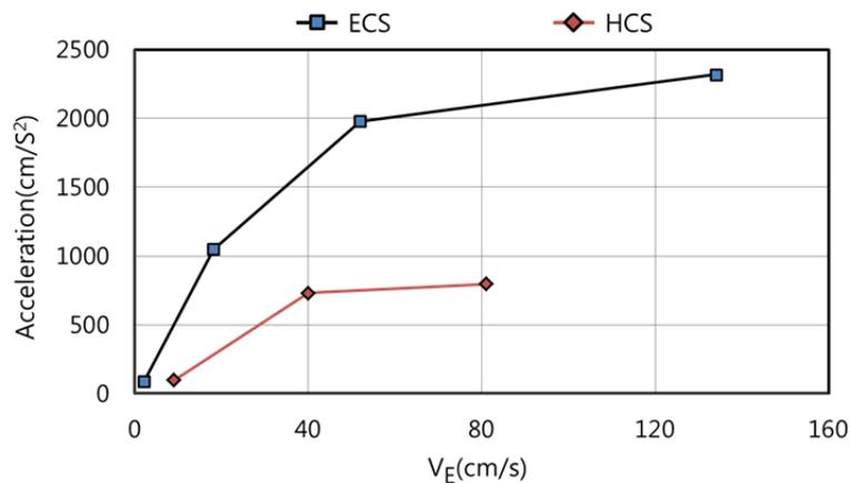
**Figure 7.** The Relation between acceleration and energy-equivalent velocity
