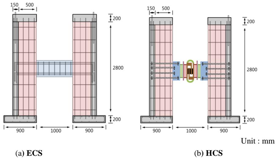
**Figure 4.** Specimen Drawings
