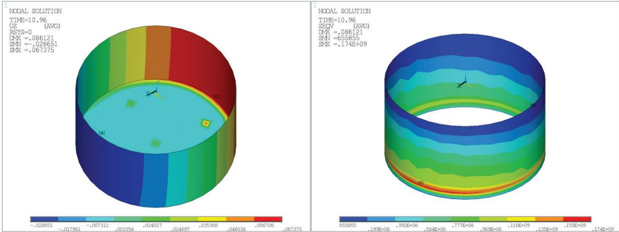
Figure 3.7. Vertical displacement (left) and Von Mises stress in shell after retrofitting
