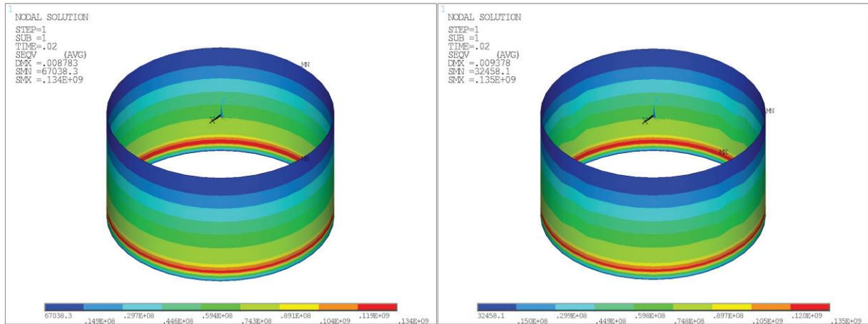
**Figure 3.1.** Von Mises stress against hydrostatic pressure in shell before (left) and after (right) retrofit
