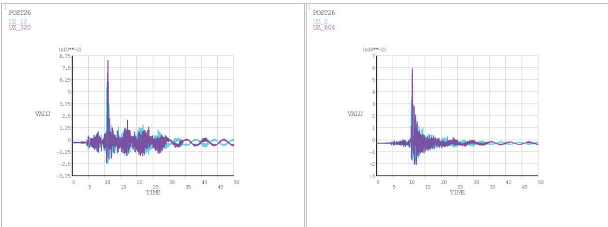
**Figure 3.5.** Non-linear dynamic (time-history) analysis results – base vertical displacement – After Retrofitting
