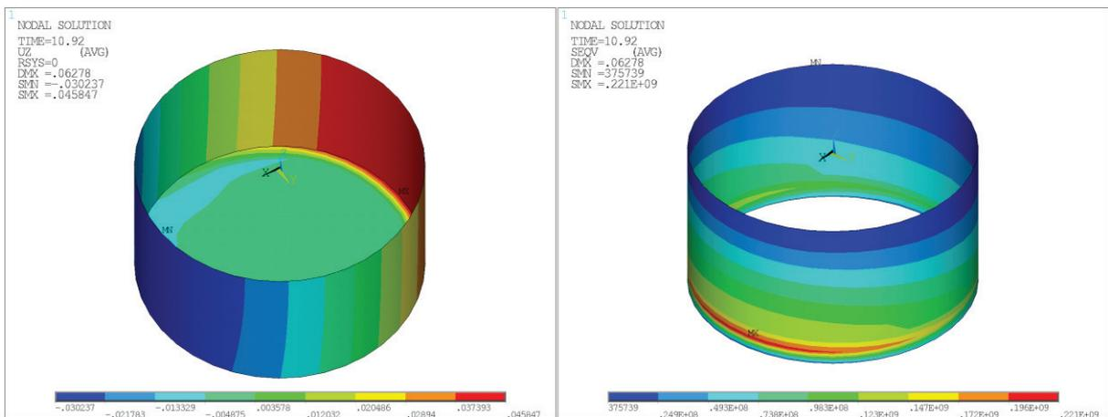
**Figure 3.6.** Vertical displacement (left) and Von Mises stress in shell before retrofitting
