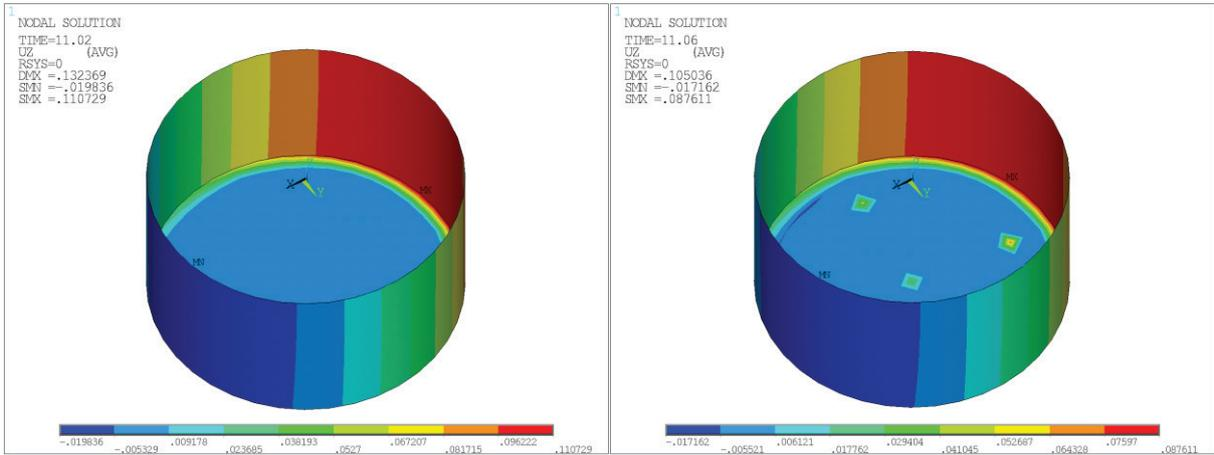
Figure 3.8. Vertical deflection in tank shell before (left) and after (right) retrofitting
