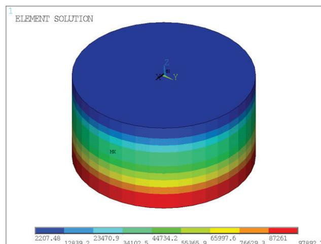
**Figure 2.1.** Hydrostatic pressure in model (Average value in element center – Unit : Pa )
