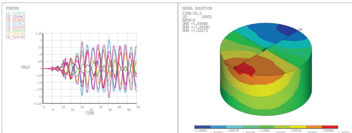
**Figure 3.3.** Liquid sloshing amplitude before retrofitting
