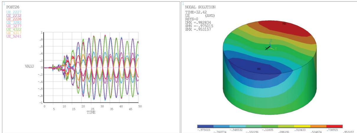
**Figure 3.2.** Liquid sloshing amplitude before retrofitting
