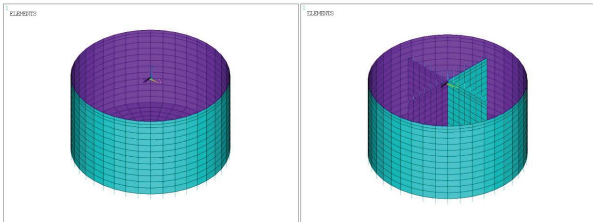
**Figure 2.2.** Isometric perspective view of the tank before (left) and after (right) retrofitting
