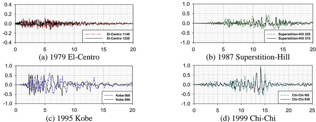
**Figure 3.1.** Ground acceleration time histories of the four ground-motions (vertical axis: ground acceleration (g); horizontal axis: time (s))
