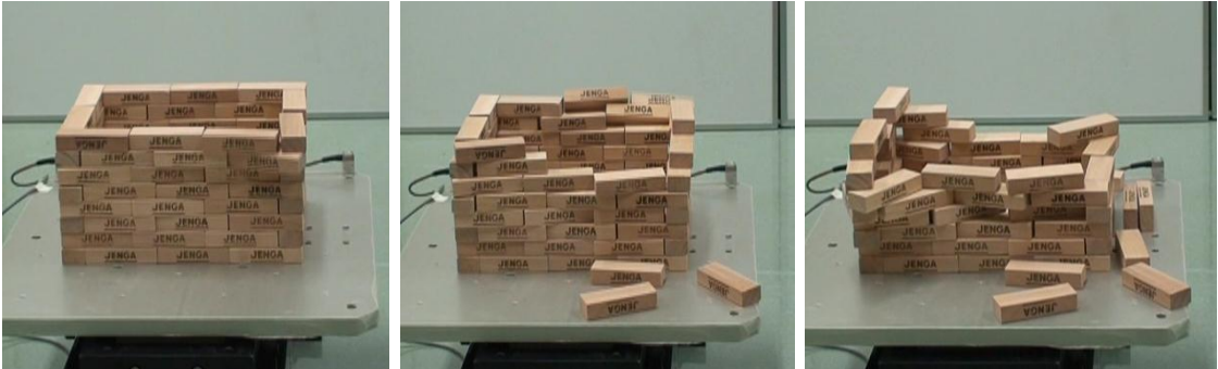
Figure 1. Collapse pattern of model 1 (length height ratio = 1.5)
