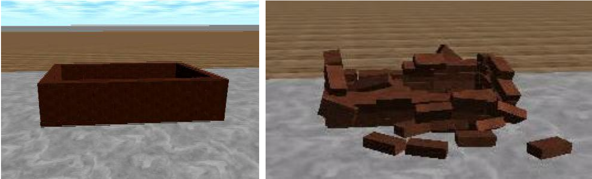
Figure 7. Collapse simulation of small specimen on small size shaking table
