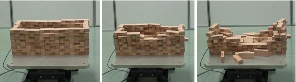
Figure 2. Collapse pattern of model 2 (length height ratio = 2.1)
