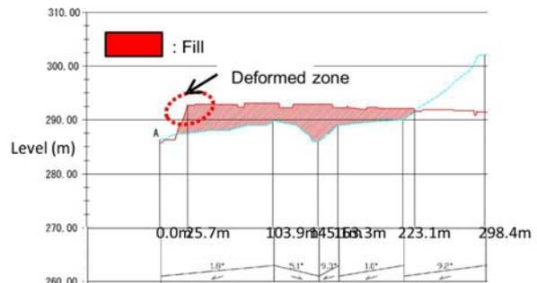
**Figure 23** Cross section
