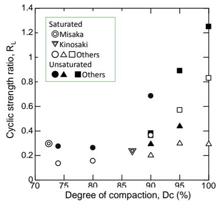
**Figure 21** Relationship between Degree of compaction and cyclic strength ratio
