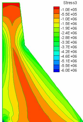
(b) Contour of compressive principle stress (case 3)
