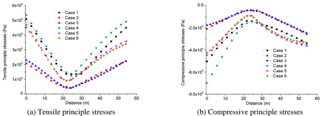
**Figure 6.4.** Stress distribution at the section 20m above the base at the Koyna dam
