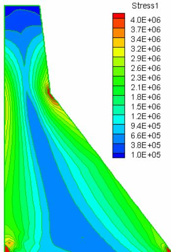
(a) Contour of tensile principle stress (case 3)
