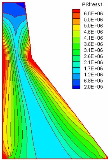
(a) Contour of tensile principle stress (case 1)
