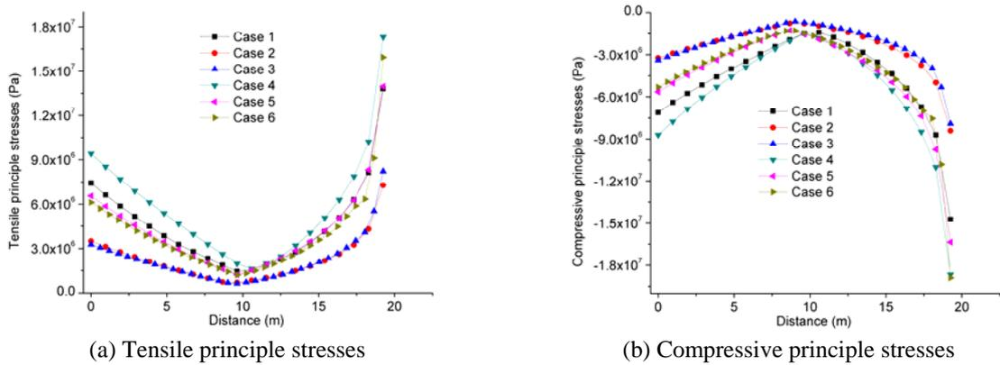
**Figure 6.3.** Stress distribution at the neck section of the Koyna dam
