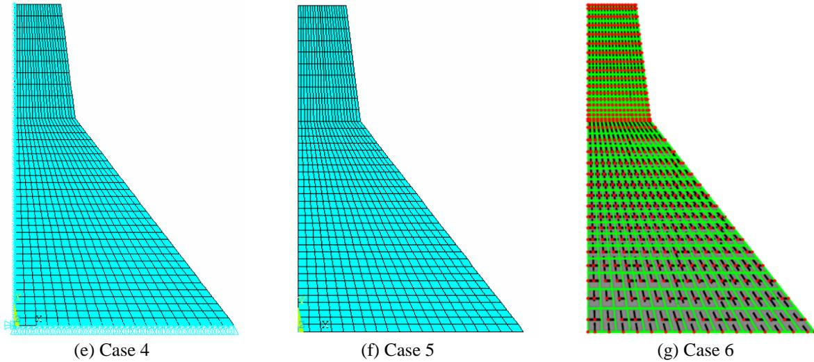
**Figure 6.2.** Koyna dam geometry and its mesh discretization
