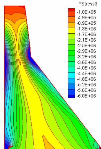
(b) Contour of compressive principle stress (case 1)
