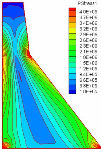
(a) Contour of tensile principle stress (case 2)
