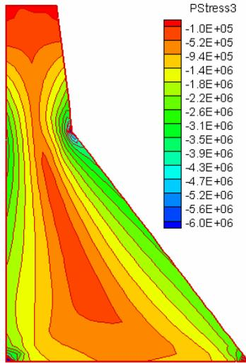
(b) Contour of compressive principle stress (case 2)
