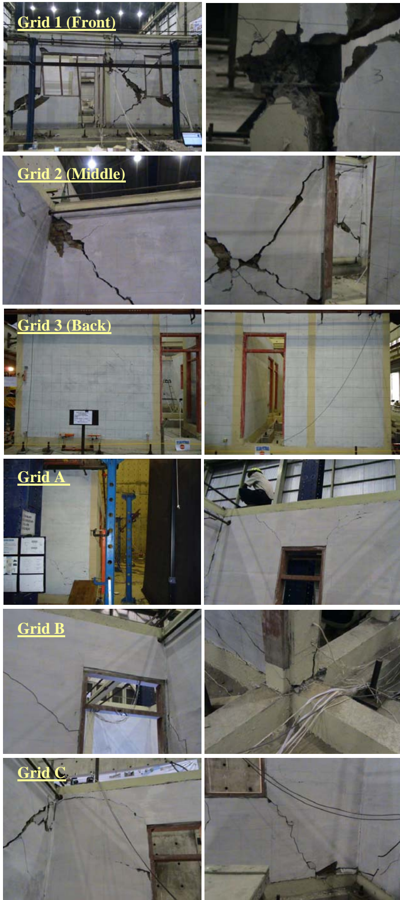
Figure 8 Damages on Non-Engineered Structural Model (Final Stage)
