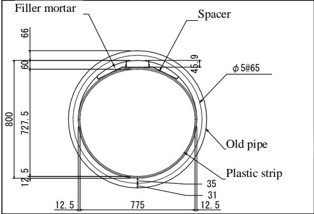
Figure 3.1. Section view of the composite pipe
