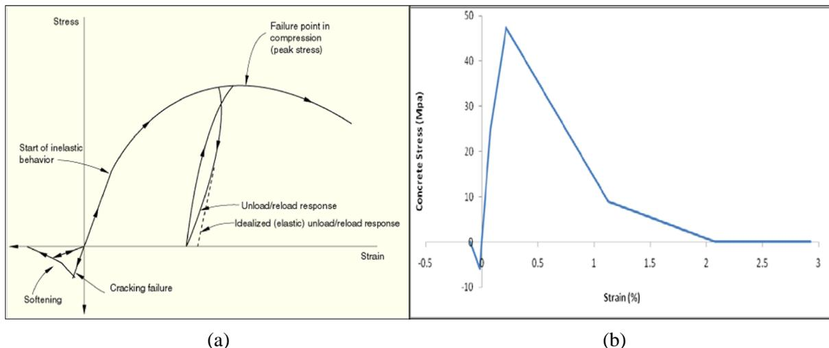
**Figure 4.3.** (a) Conceptual hysteretic model and (b) nonlinear behaviour of concrete
