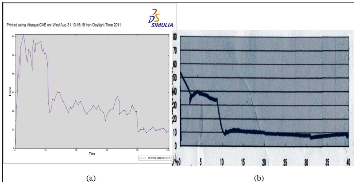
**Figure 5.2.** Total applied pull-out force by (a) simulation and (b) experimentation
