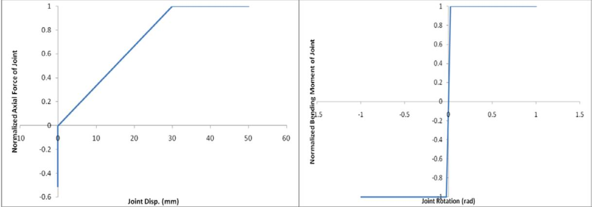
**Figure 4.4.** Joint behaviour of RC pipes (normalized values)
