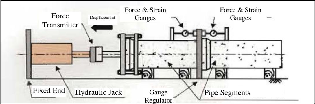
Figure 3.2. Schematic outline of the experimental setup [Takada & Kuwata, 2010]
