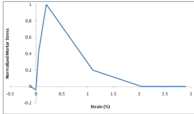
**Figure 4.6.** Nonlinear behaviour of high strength mortar
