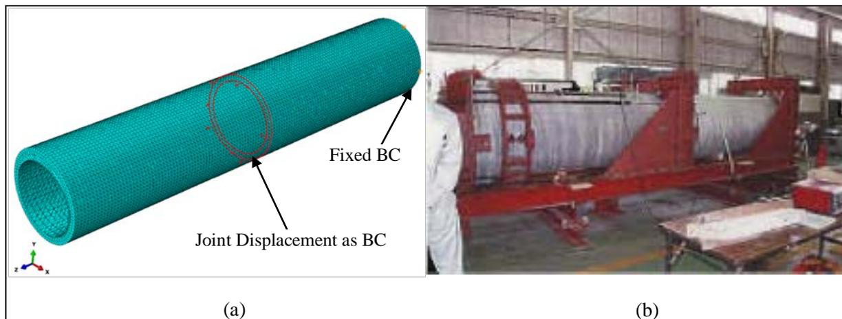
**Figure 5.1.** (a) Boundary conditions applied to the FE model, (b) Loading conditions in the experimentation [Takada & Kuwata, 2010]
