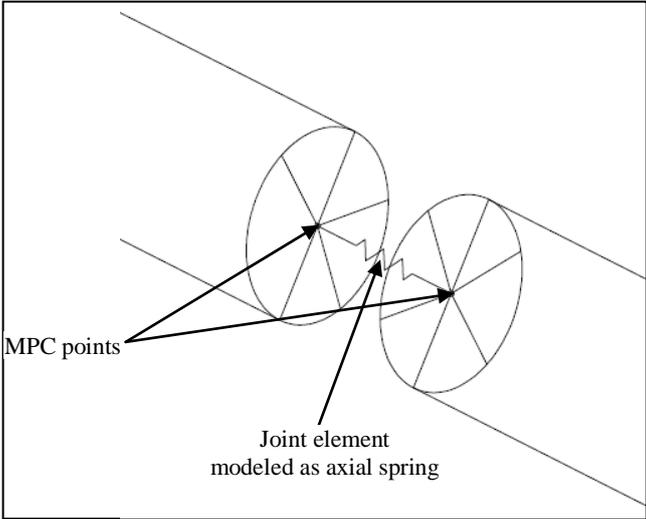
**Figure 4.5.** Concept of proposed model for pipe joint (the spacing scale is exaggerated)
