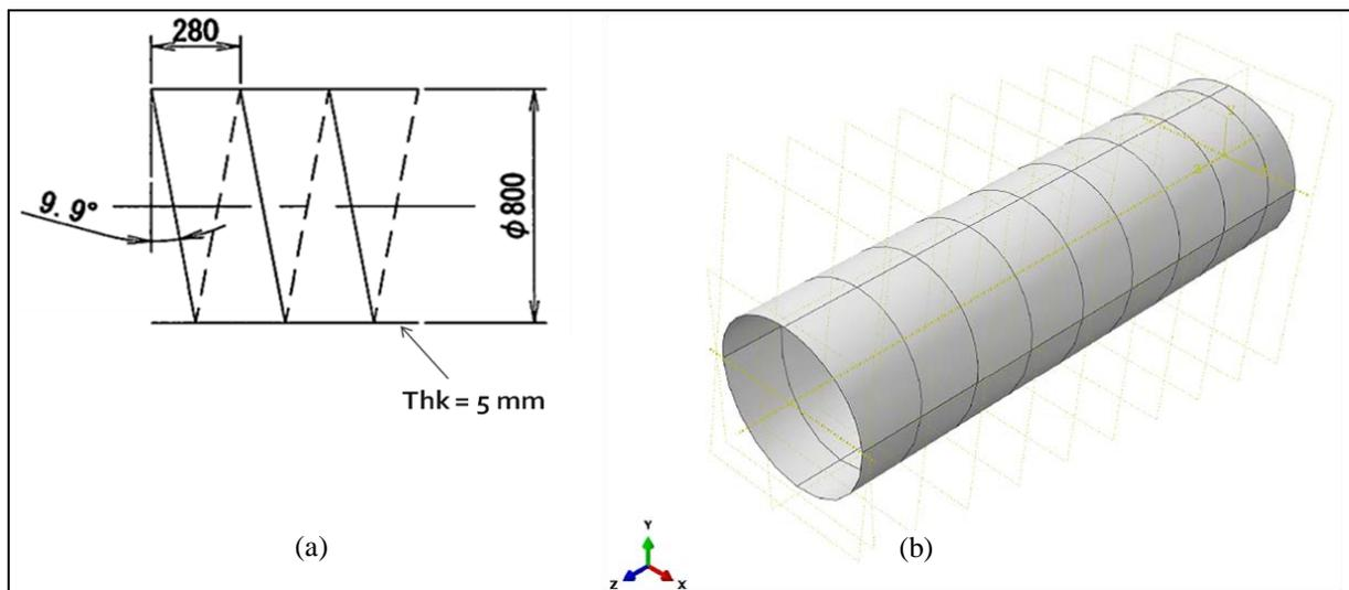
**Figure 4.1.** (a) Geometrical dimensions, (b) physical model of the jointed inserted pipe
