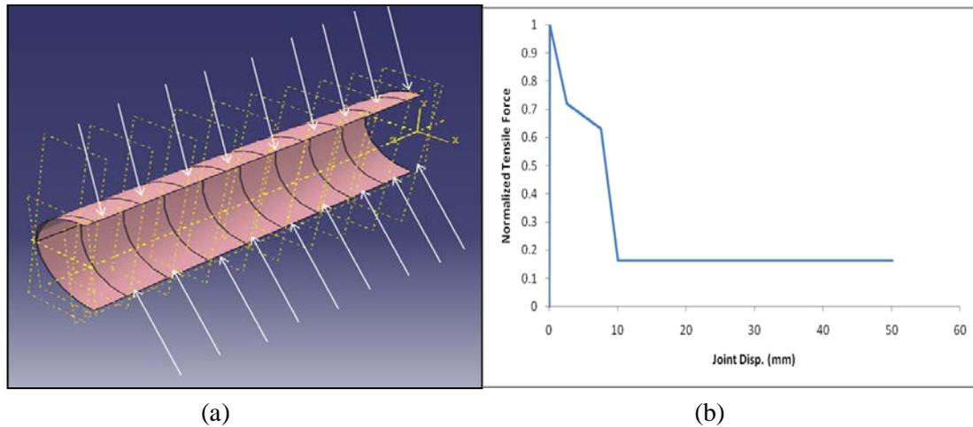
**Figure 4.2.** (a) Joint locations of the inserted pipe, (b) Normalized tensile strength of inner pipe joints
