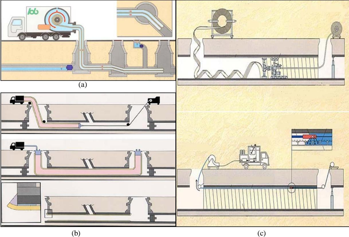
**Figure 2.1.** Rehabilitation of sewer pipelines by (a) reverse pipe method, (b) pipe formation method and (c) composite pipe method
