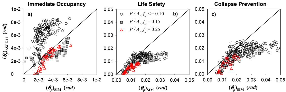
**Figure 4.** Comparison of calculated plastic rotation limits with the ASCE/SEI 41 limits
