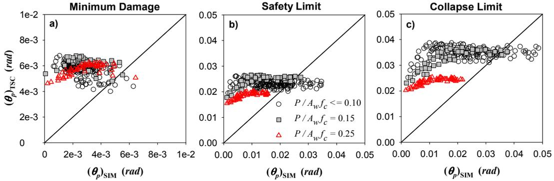
**Figure 6.** Comparison of calculated plastic rotation limits with the TSC-07 limits
