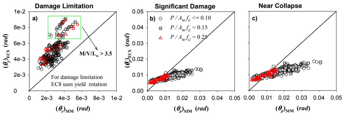
**Figure 5.** Comparison of calculated plastic rotation limits with the plastic chord rotation limits in EC8-3
