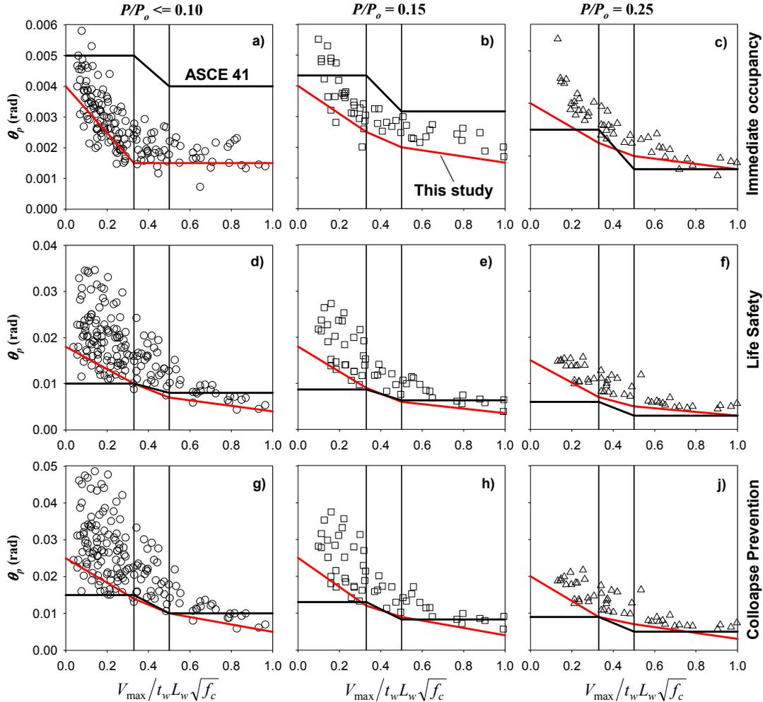
**Figure 7.** Lower bound plastic rotation limits at different performance levels
