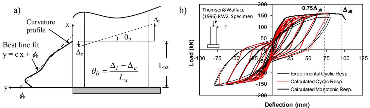
**Figure 3.** a) Schematic descriptions of base curvature and rotation calculation, b) Typical load-deformation curves of analyzed wall models
