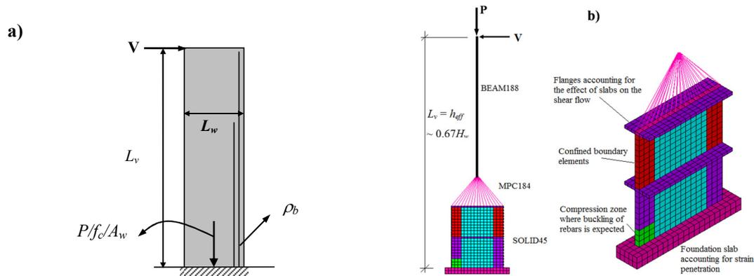
**Figure 2.** a) Illustration of variables of the parametric study; b) Finite element model.
