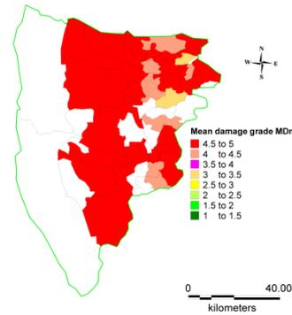
**Figure 4.10.** Damage scenario for 3 m flood height
