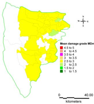
**Figure 4.7.** Damage scenario for 0.5 m flood height
