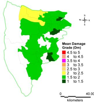
**Figure 4.3.** Mean Damage Grade ( $D_m$ ) for an assumed  $I_0=XI$ , 1935 Quetta earthquake
