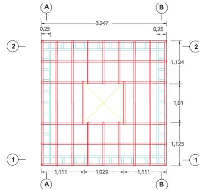
Wooden roof configuration (Crown beam shown in blue)
