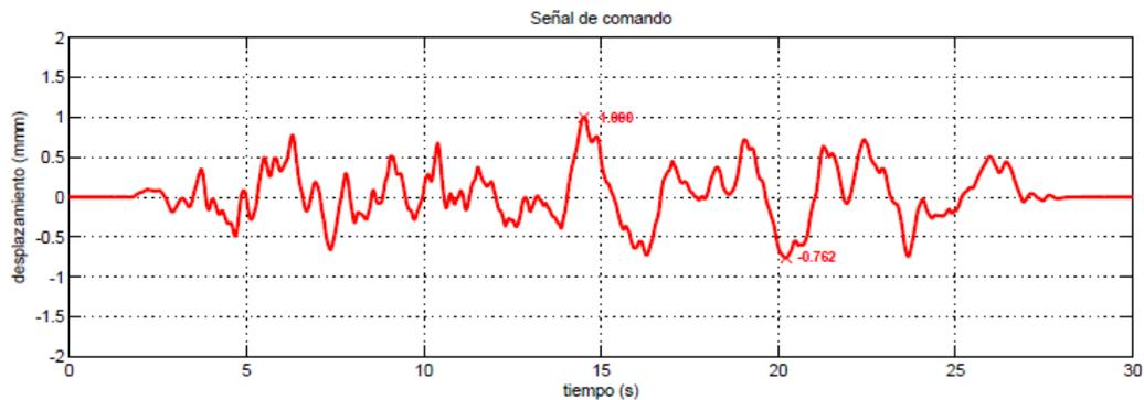
**Figure 3.** Shaking table command displacement (normalized to 1 mm).
