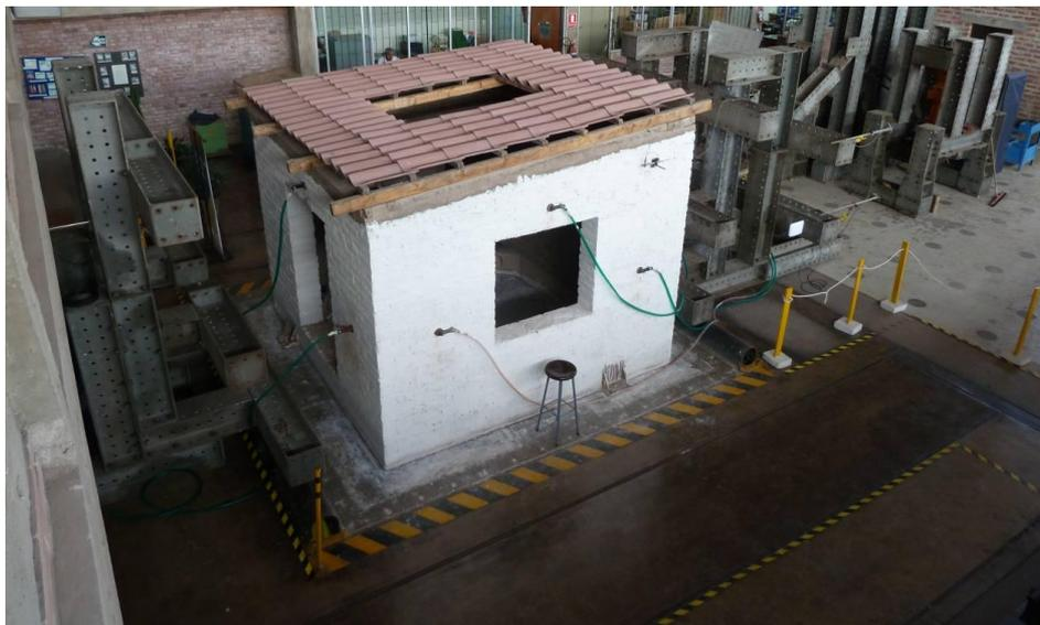
**Figure 5.** Full-scale model on shaking table
