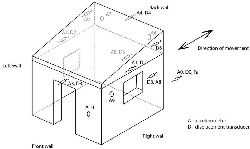
**Figure 4.** Instrumentation location
