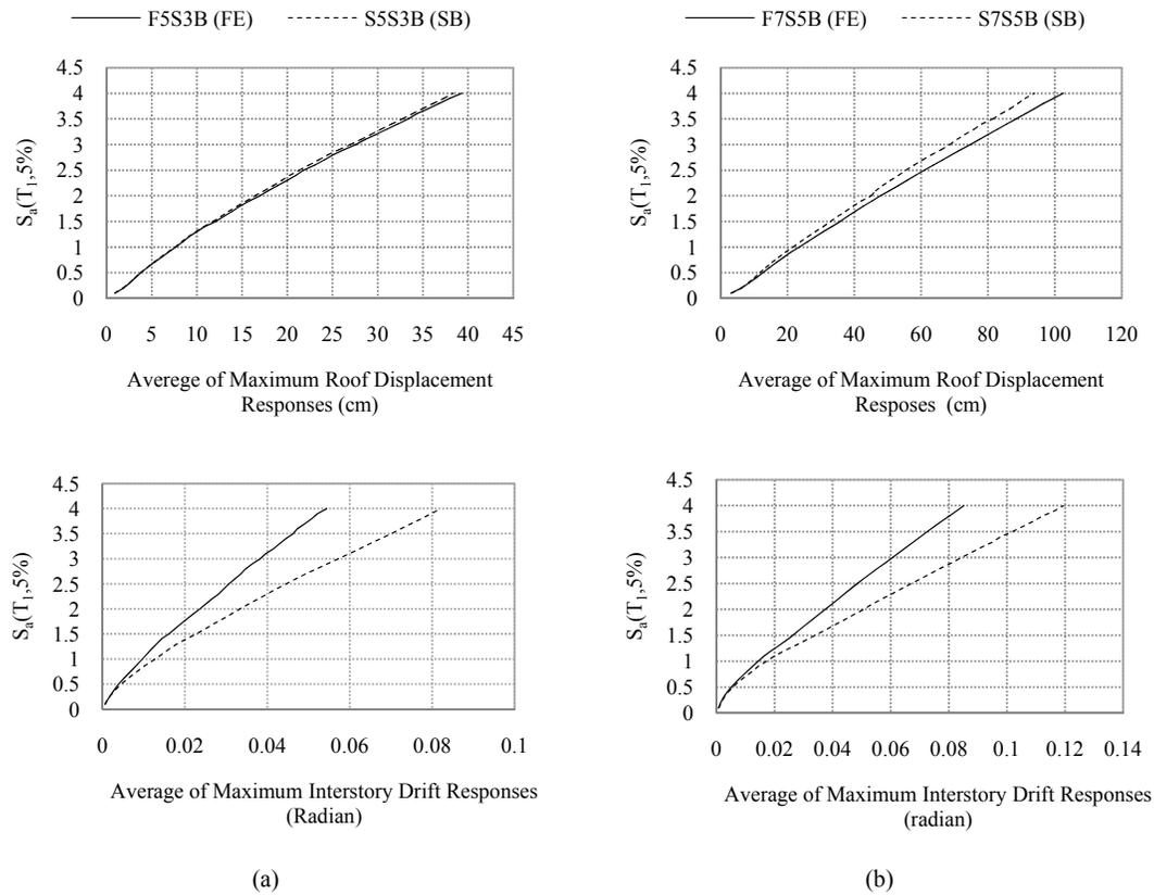
**Figure 3.2.** Comparing the averages of maximum roof displacement responses and maximum interstory drift in IDA analyses of the models: (a) F5S3B, S5S3B; (b) F7S5B and S7S5B; under 19 selected records
