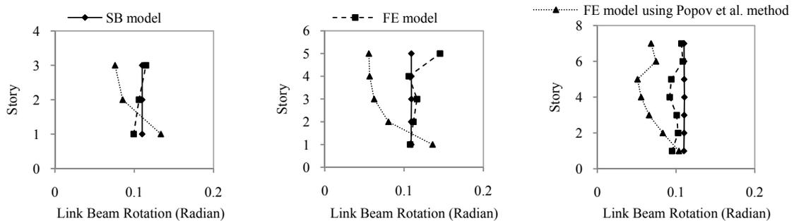
**Figure 4.2.** The average maximum link beam rotations over the frame's height, analyzed subjected to 7 records
