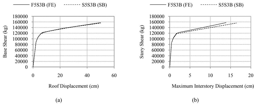
**Figure 3.1.** Comparing the responses obtained from pushover analysis of models F5S3B and its equivalent shear building (S5S3B): a) roof displacement; b) maximum interstory displacement
