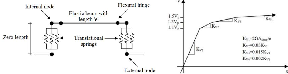
**Figure 2.2.** (a): EBF link element; (b): Combined behavior of parallel translational springs
