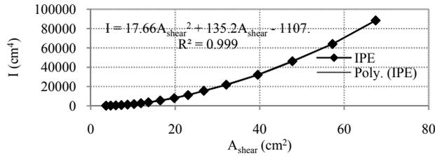
**Figure 4.1.** The relation between the beam moment of inertia and the beam shear area for IPE sections
