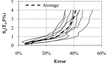
**Figure 3.3.** The error of SBMs in estimating the mean maximum interstory drift
