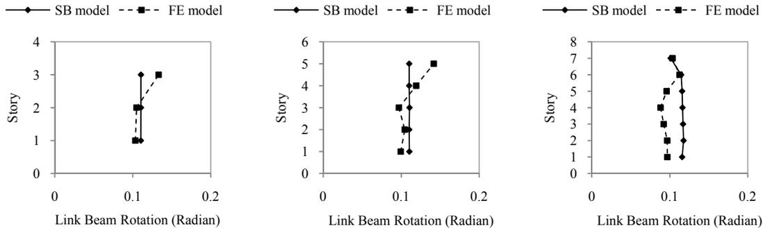
**Figure 5.1.** The average of maximum link beam rotations over the height of frames analyzed by 3 acc. functions
