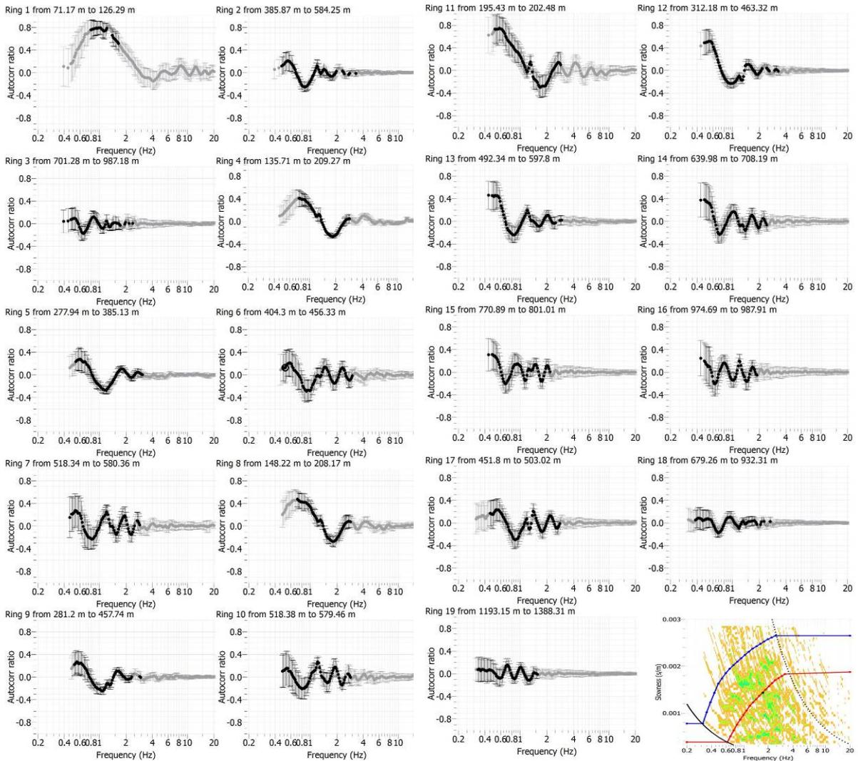
Figure 6 : Auto correlation ratio curve for all arrays
