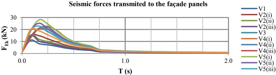
Figure 4.3. Maximum seismic force transmitted to the panels
