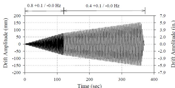
**Figure 2.2.** Displacement time history for dynamic crescendo test (AAMA 2009)
