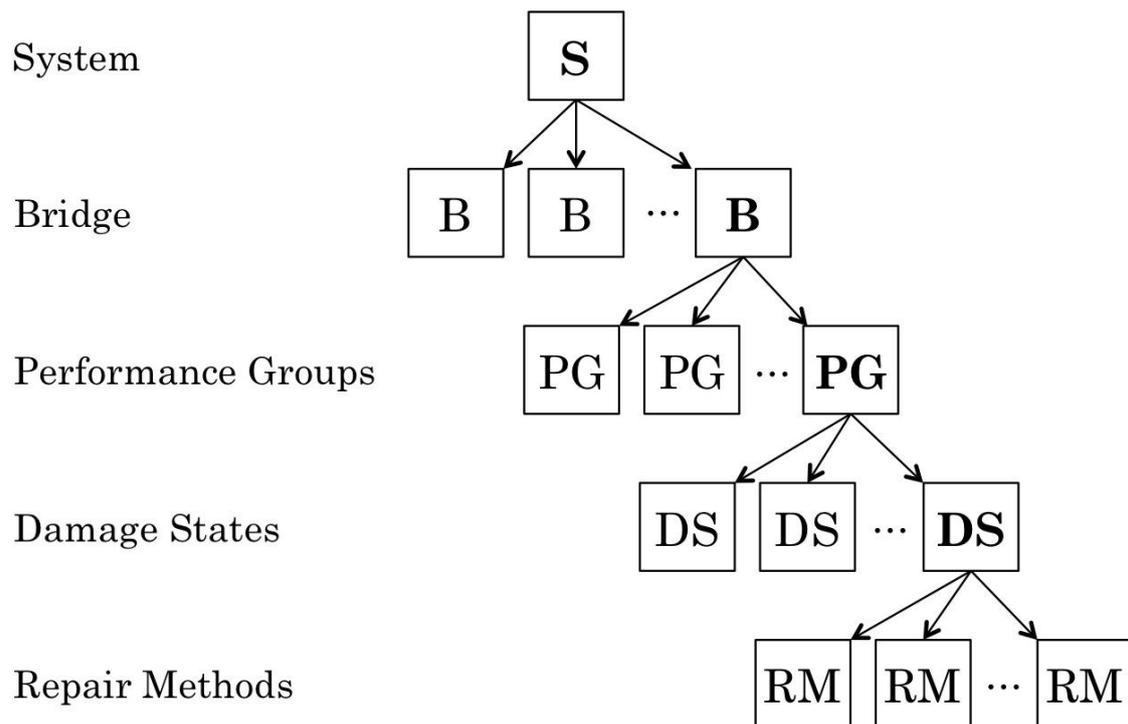
**Figure 1.** Example branch of the PEER PBEE Framework Structure after Mackie et al. 2007
