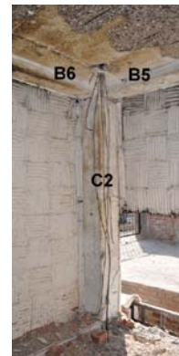
(b) Frame sub-assembly after fire test
