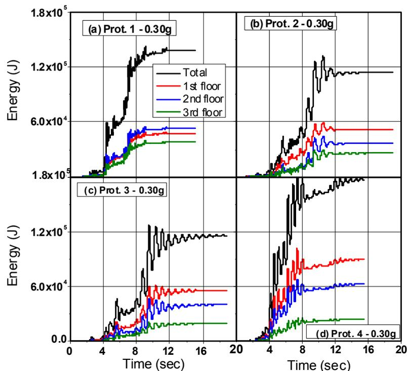
**Figure 8.** Total and cumulative energies dissipated in each floor at PGA of 0.30g, for: (a) Prototype 1. (b) Prototype 2. (c) Prototype 3. (d) Prototype 4.
