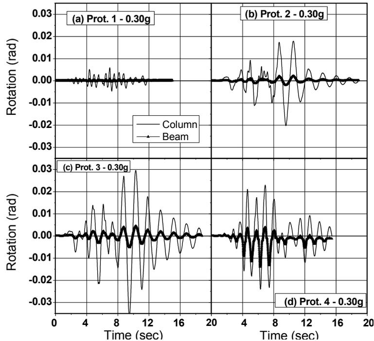
**Figure 7.** Evolution of column and beam rotation in first floor's joint at PGA of 0.30g for: (a) Prototype 1. (b) Prototype 2. (c) Prototype 3. (d) Prototype 4.
