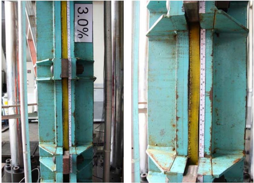
Figure 3.2. Experimental observations of the high mode buckling wave length
