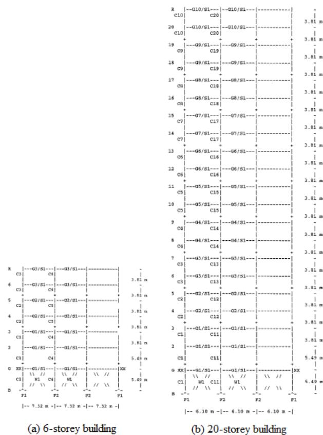
**Figure 3.** Finite element models of the 6-storey and 20-storey buildings
