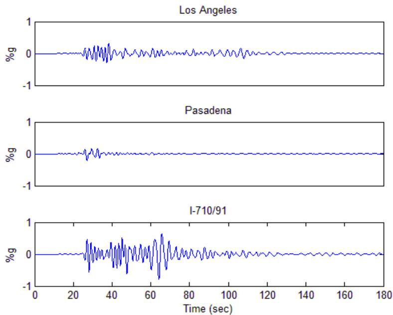
**Figure 4.** Ground motions for different building sites due to a M6 earthquake at San Bernardino with dip=  $90^\circ$ , rake=  $180^\circ$ , and strike =  $120^\circ$
