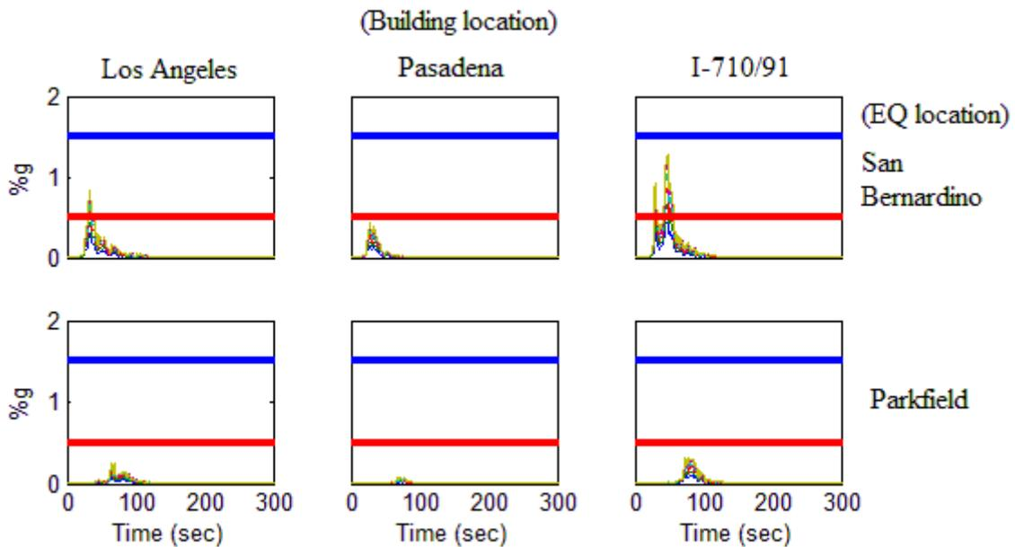
**Figure 7.** Seismic shaking level for 6-storey building. 6 curves on each plot correspond to different floor acceleration responses. (Red line: threshold for minor shaking; Blue line: threshold for moderate shaking)
