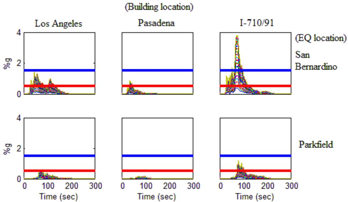
**Figure 6.** Seismic shaking level for 20-storey building. 20 curves on each plot correspond to different floor acceleration responses. (Red line: threshold for minor shaking; Blue line: threshold for moderate shaking)
