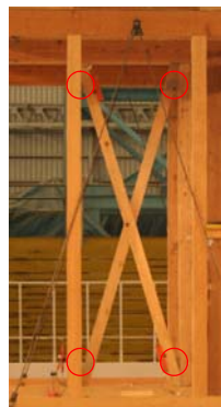
Picture 1. Wood brace fastened by the new fastener
