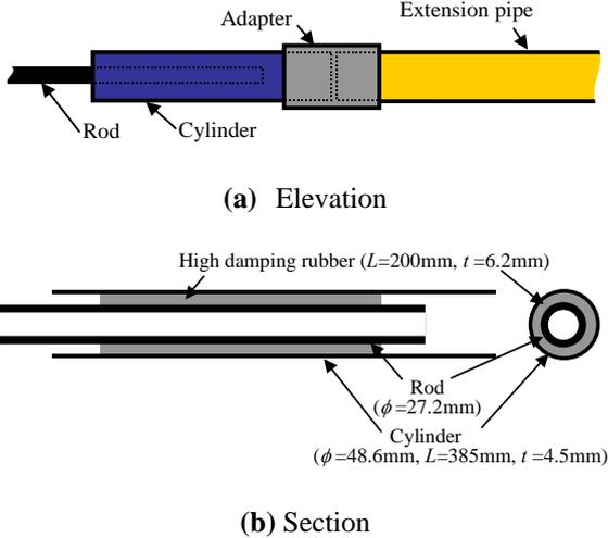
**Figure 2.1.** Cylindrical Damper and Adapter
