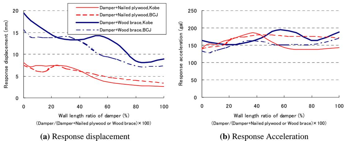
**Figure 5.9.** Relationship between Response of Frame and Wall Length Ratio of Damper
