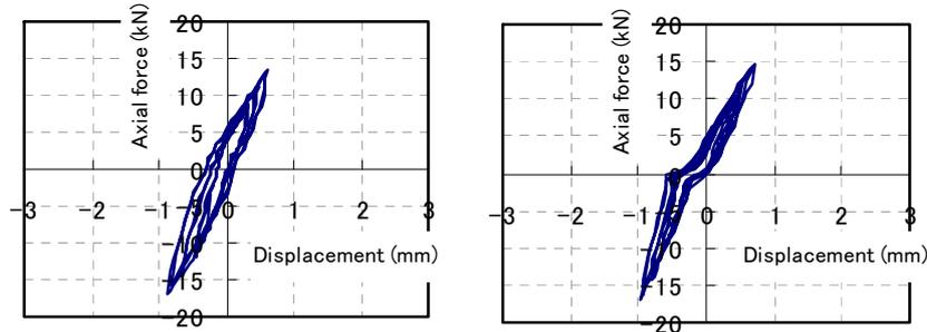
**(a)** Total Slip of Two End Joints of Upper Damper    **(b)** Total Slip of Two End Joints of Lower Damper
