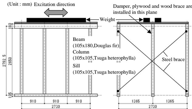
Figure 3.1. Elevations of the Three Wood Frames for Shaking Table Tests
