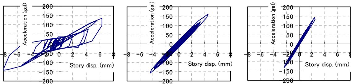
(a) Wall length ratio of damper=0% ( $K_1=4.97$ ,  $K_2=2.86$  kN/cm) (b) Wall length ratio=50% ( $K_1=9.11$ ,  $K_2=4.67$  kN/cm) (c) Wall length ratio=100% ( $K_1=13.25$ ,  $K_2=6.48$  kN/cm)
