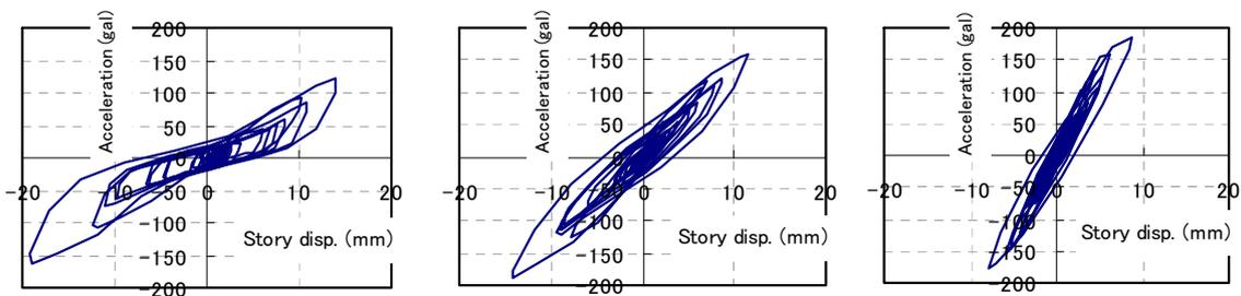
(a) Wall length ratio of damper=0% ( $K_1=3.48$ ,  $K_2=3.27$  kN/cm) (b) Wall length ratio=50% ( $K_1=8.37$ ,  $K_2=4.88$  kN/cm) (c) Wall length ratio=100% ( $K_1=13.25$ ,  $K_2=6.48$  kN/cm)
