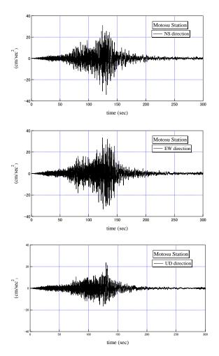
Figure 3.1. Accelerorams of recorded ground motions at Motosu K-NET observation station
