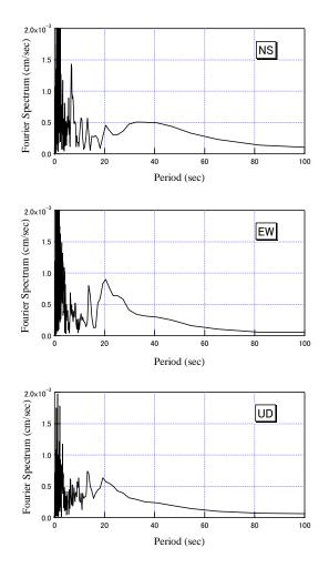
Figure 3.2. Fourier spectra of recorded ground motions at Motosu K-NET observation station
