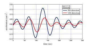
**Figure 5.3.** Superposition of acceleration time histories of NS and UD components of the observed ground motions processed by a low-pass filter with a period, 50 seconds
