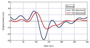
**Figure 5.2.** Superposition of displacement time histories of NS and UD components of the observed ground motions processed by a low-pass filter with a period, 50 seconds
