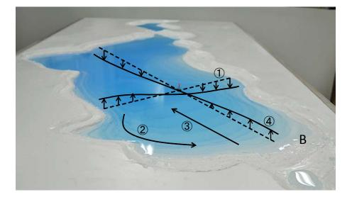
**Photograph 6.1.** Saiko model and description of mechanism on seismic seiche came up in Lake Saiko (Point B in the photograph is correspondent with the location of Point B in Figure 1.1)
