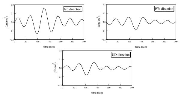
Figure 5.1. Accelerograms of the observed ground motions processed by low-pass filter with a period, 50 seconds.
