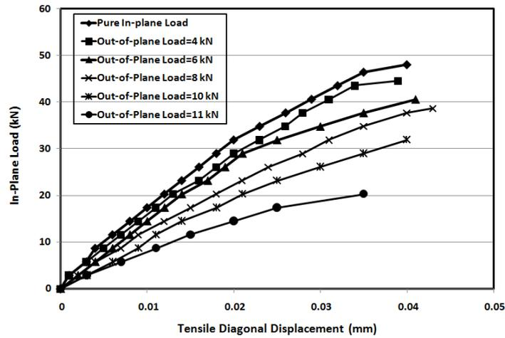
Figure 5. Average in-plane load-displacement curves for different in-plane, out-of-plane load combinations
