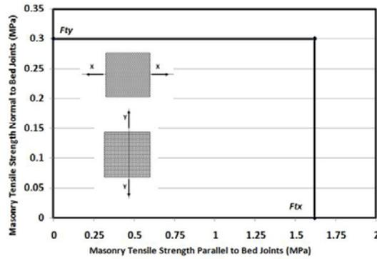
Figure 9. Rankin's failure criteria for brickwork (principal direction along the bed joints)
