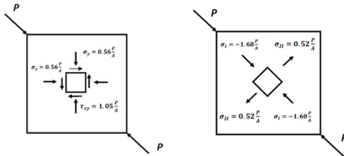
Figure 7. Stress state in a square plate subjected to compressive diagonal force
