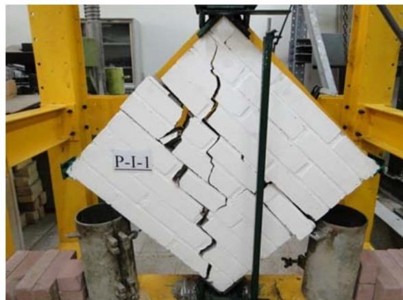
Figure 2. Typical failure of the wall panels under in-plane shear load
