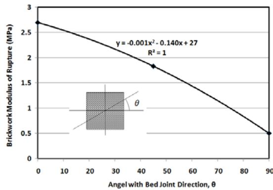
Figure 10. Brickwork modulus of rupture in different directions
