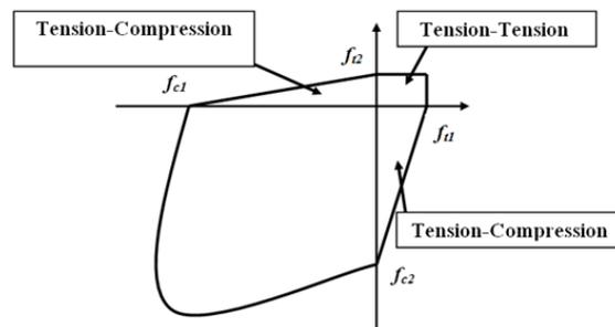
Figure 8. General shape of the applied failure criterion
