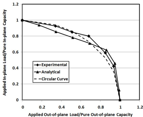
Figure 12. Comparison of the in-plane, out-of-plane capacity interaction curves for brick masonry
