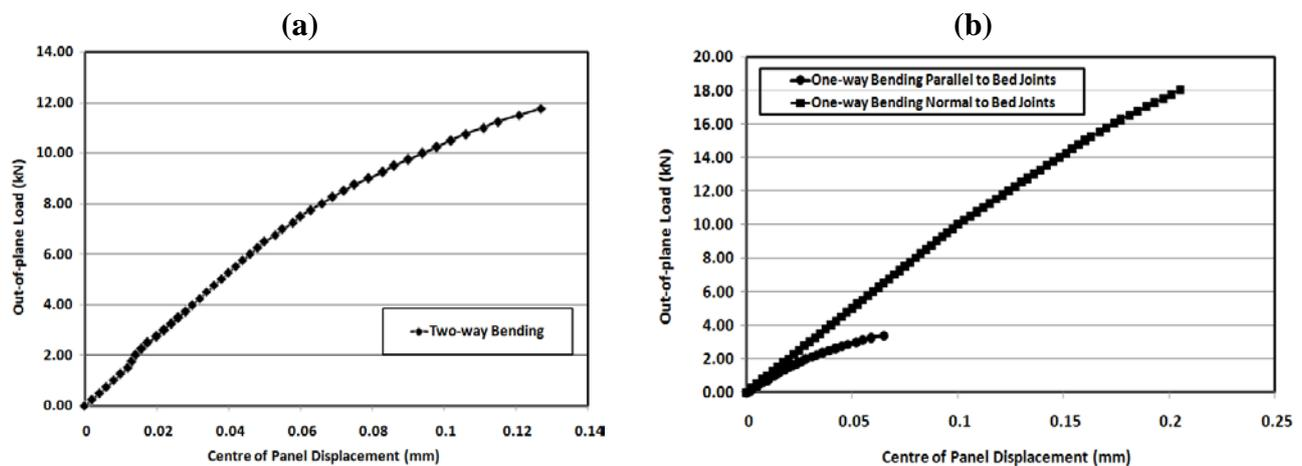
Figure 4. Average out-of-plane load-displacement curves; (a) two way bending, (b) one way bending
