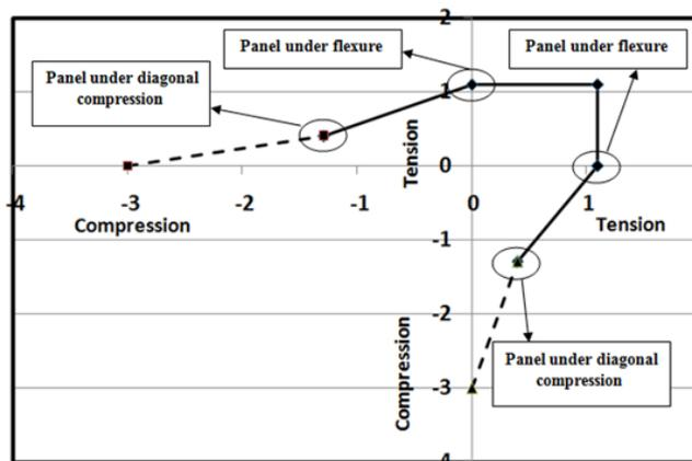
Figure 11. Proposed failure criteria for the combined in-plane, out-of-plane loading (principal direction at 45 degrees to the bed joints)
