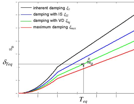
**Figure 3.** Equivalent spectral damping
