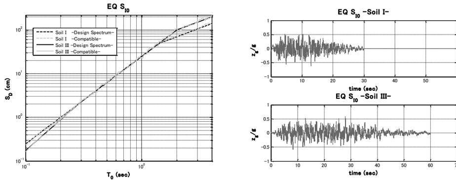
**Figure 4.** Artificial earthquakes compatible with the displacement spectra
