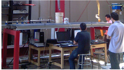
Figure 6. Single span bridge model
