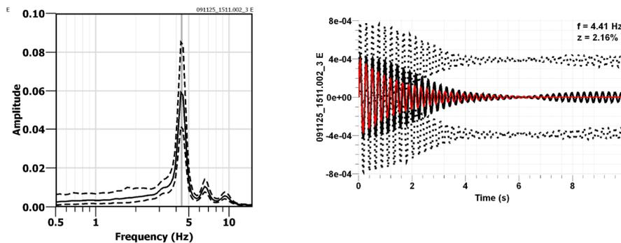
**Figure 4.2.** Frequency and damping of the house after strengthening
