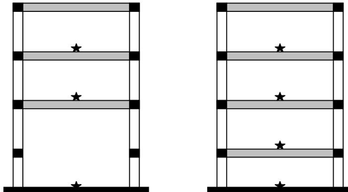
**Figure 3.1.** Instrumentation schemes, left before strengthening, right after strengthening,
