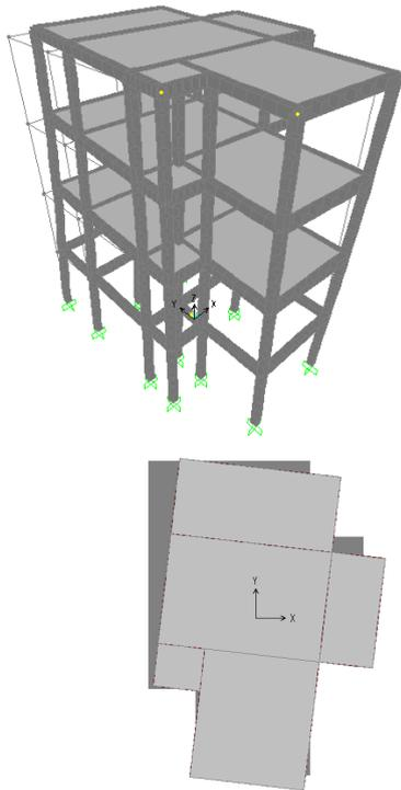
**Figure 7.1:** 1<sup>st</sup> vibration mode (torsion) of the initial structure
