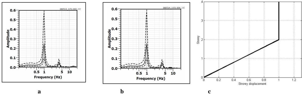
**Figure 6.1:** building modal shape before strengthening: (a) and (b) displacement amplitude of inhabitable storeys, (c) modal shape
