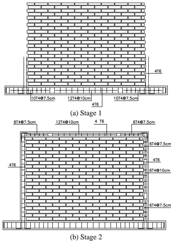
**Figure 2.** Confined masonry wall construction stages
