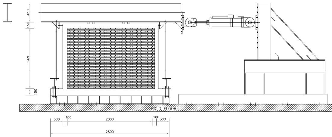
**Figure 4.** Loading setup
