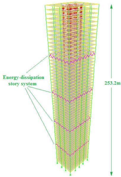
**Figure 1.** 3D building elevation
