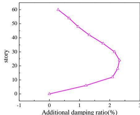
**Figure 6.** Top floor displacement of various models **Figure 7.** Additional damping ratio of various models
