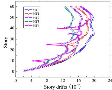
**Figure 8.** Displacement of basic model arrangements **Figure 9.** Story drifts of basic model arrangements
