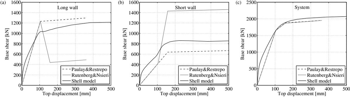
**Figure 4.4.** Force-deformation relationships of the coupled individual walls and of the system: comparison of numerical results obtained with the shell element model and the two analytical models.
