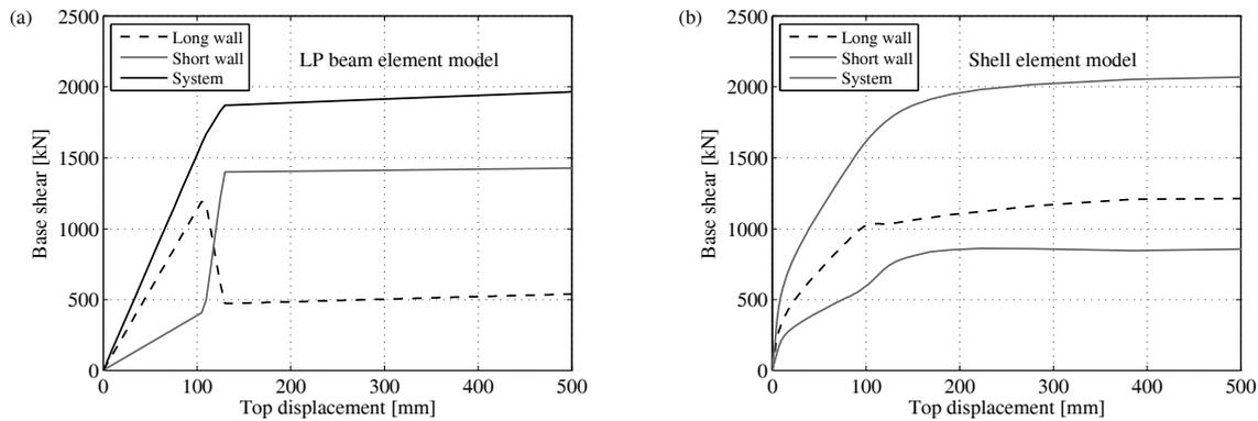
**Figure 4.5.** Comparison of the force-deformation relationships obtained for the coupled system with the numerical models: (a) lumped plasticity beam element model, (b) shell element model.
