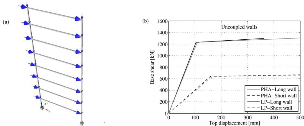
**Figure 4.1.** (a) Screenshot of the coupled wall system with the lumped plasticity model in Seismostruct. (b) Force-deformation relationships of the single walls obtained: Comparison of the results obtained with the numerical model and the results obtained from the plastic hinge analysis.
