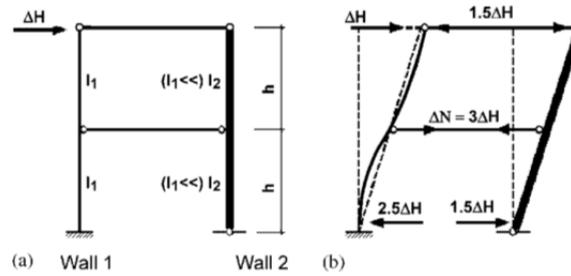
**Figure 3.2.** Two storey system: (a) Properties and loading, (b) assumed deflected shape and resulting floor forces and base shear forces (Rutenberg, 2004).
