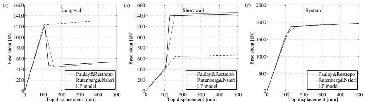
**Figure 4.2.** Force-deformation relationships of the coupled individual walls and of the system: comparison between numerical results obtained with the lumped plasticity beam element model (LP model) and the two analytical models.
