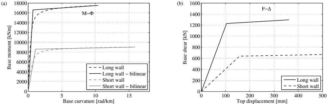
**Figure 2.2.** (a) Moment-curvature relationship of the individual walls including the corresponding bi-linear approximations. (b) Force-deformation relationship of the individual walls.
