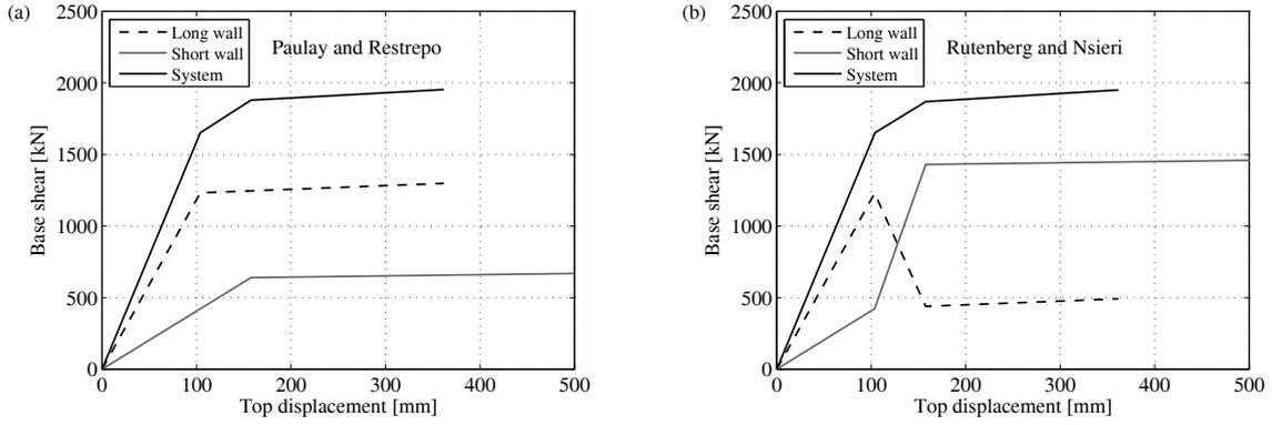
**Figure 3.1.** Force-deformation relationship of the long and short wall and of the system derived using two analytical models: (a) Paulay and Restrepo, (b) Rutenberg and Nsieri.
