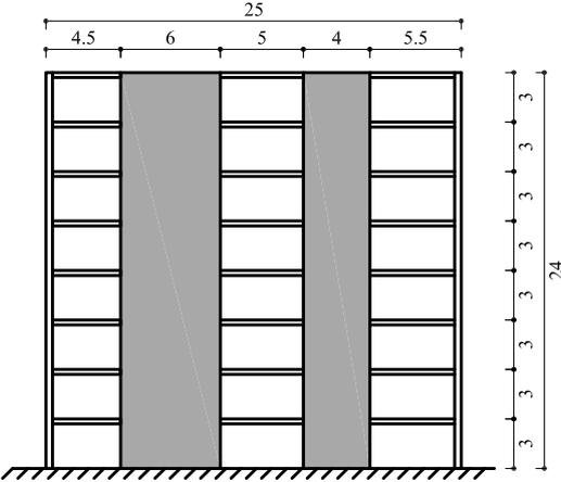
**Figure 2.1.** Geometry of the planar example structure comprising two walls of different length. All dimensions are in *m*.
