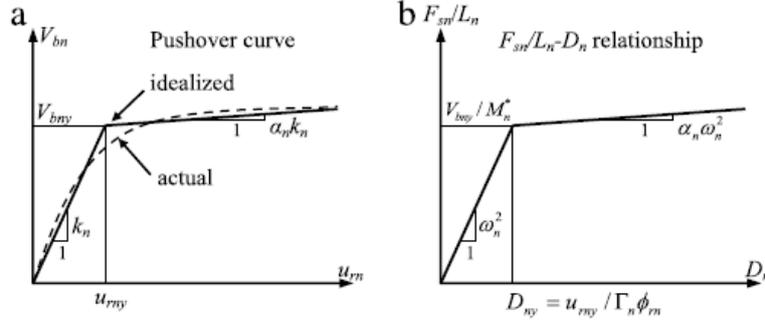
**Figure 2.1.** (a) Pushover curve and (b) force and deformation relationship of SDF system
