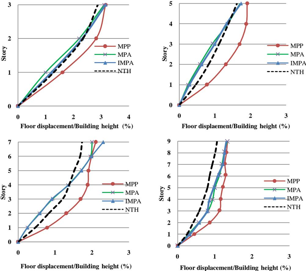
**Figure 5.1.** Median floor displacements of 3-, 5-, 7- and 9-story BRBF buildings determined by one 'mode' pushover analysis, MPA, IMPA, MPP and NTH
