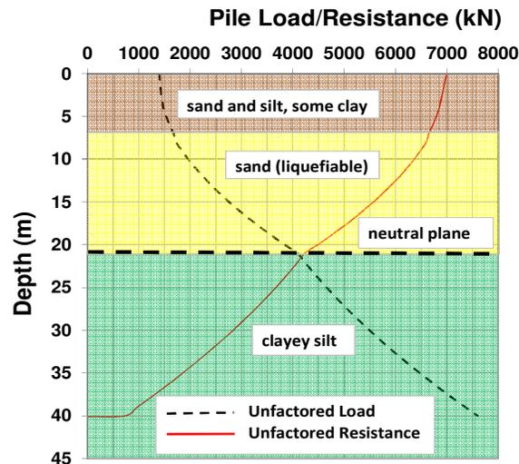
Figure 10. Axial pile design load and resistance curves (note, static neutral plane below liquefiable soils)
