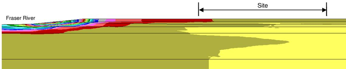
**Figure 8.** Example of relative horizontal displacement contours (contour interval = 0.1m)
