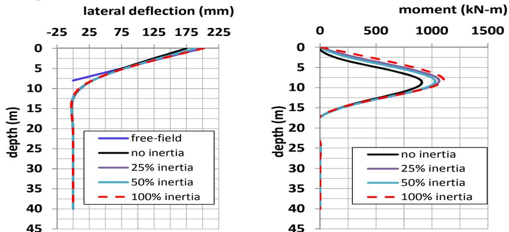
**Figure 12.** Seismic lateral pile design analyses: a) deflection and b) moment
