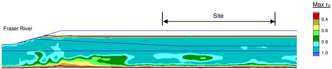
**Figure 7.** Example of maximum excess pore pressure ratios in liquefiable zones above elevation -20.5 m (2X vertical scale exaggeration)
