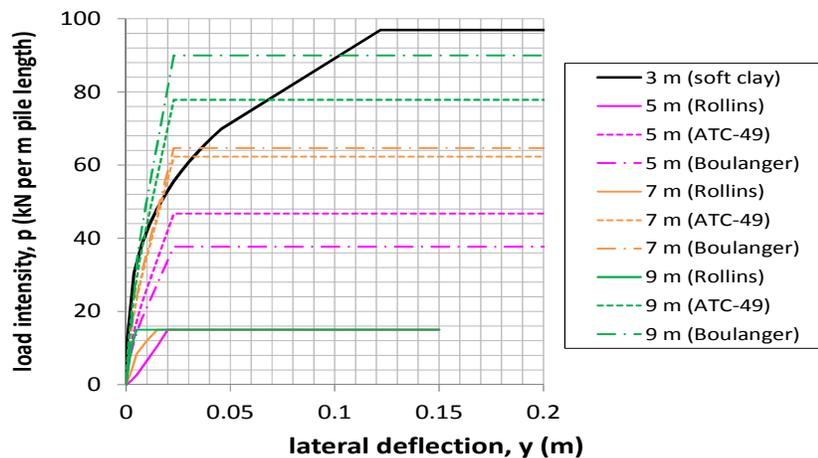
Figure 11. p-y curves at selected depths for different methods
