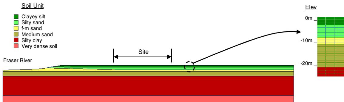
**Figure 6.** Cross-Section of FLAC model showing soil units
