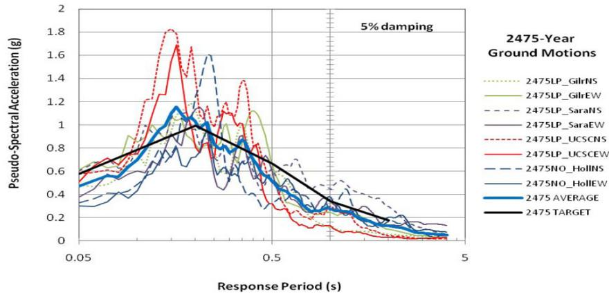
**Figure 4.** Response Spectra of Selected (Unscaled) Ground Motions (2,475 yr)
