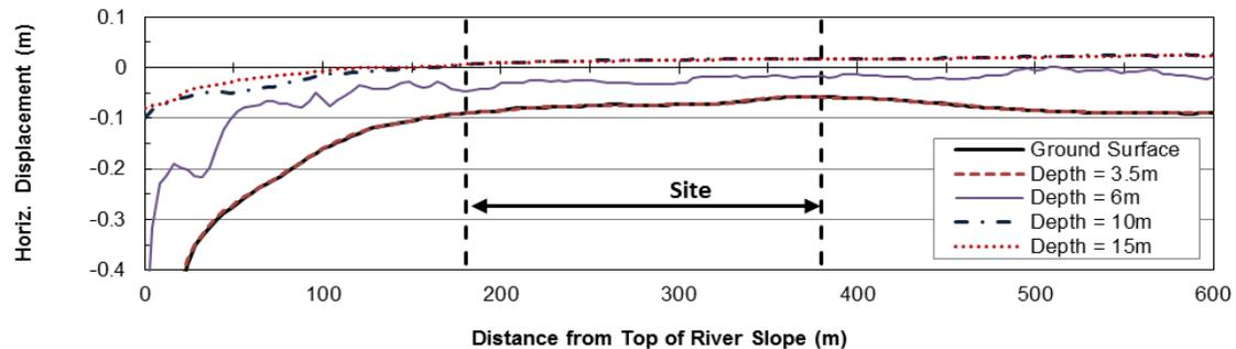
**Figure 9.** Median estimate of permanent horizontal displacement for selected depths
