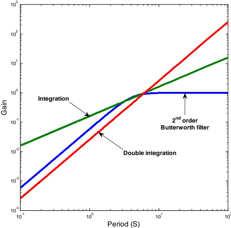
**Figure 5.** Gain function of 2<sup>nd</sup> order Butterworth filter and integration
