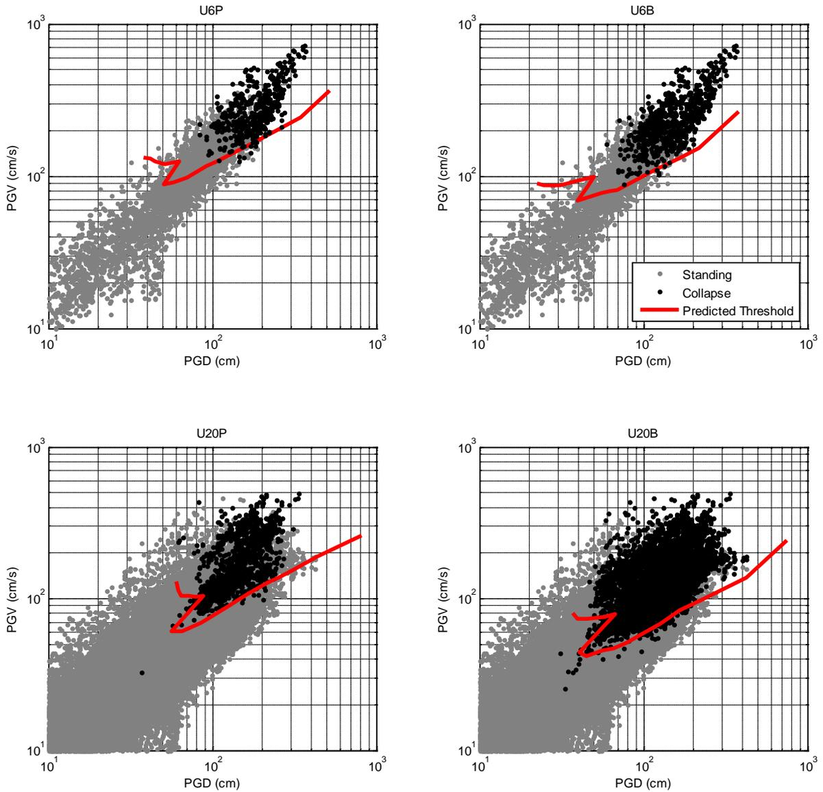
**Figure 4.** Comparison of predicted collapse thresholds and Olsen's computed results
