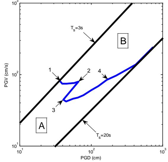
**Figure 2.** Example of collapse threshold in terms of PGV and PGD of the same building in Figure 1.
