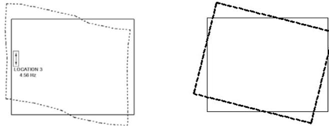
**Figure 6.2** Apparent Mode Shape 3 (AMS 3) and the Rigid-Body Approximation
