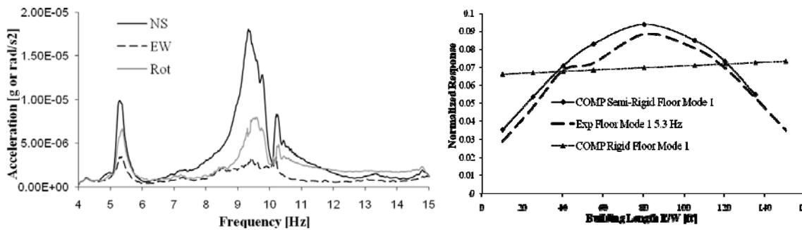
(a) Fast Fourier Transform (b) Mode 1 diaphragm deflected shape
