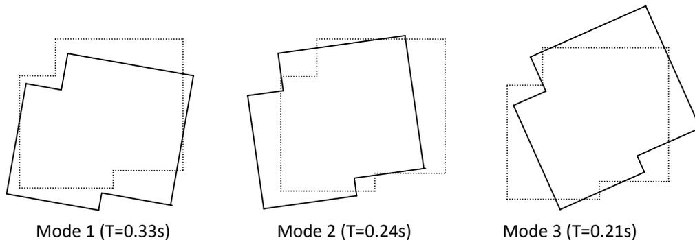
**Figure 3.2.** Experimentally determined mode shapes
