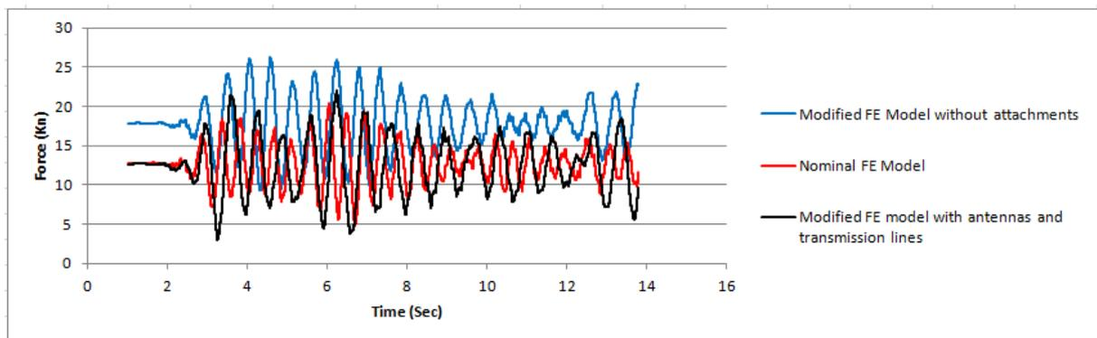
**Figure3.3.** Axial tension in a typical cable of Cluster #1 aligned with the input ground motion.
