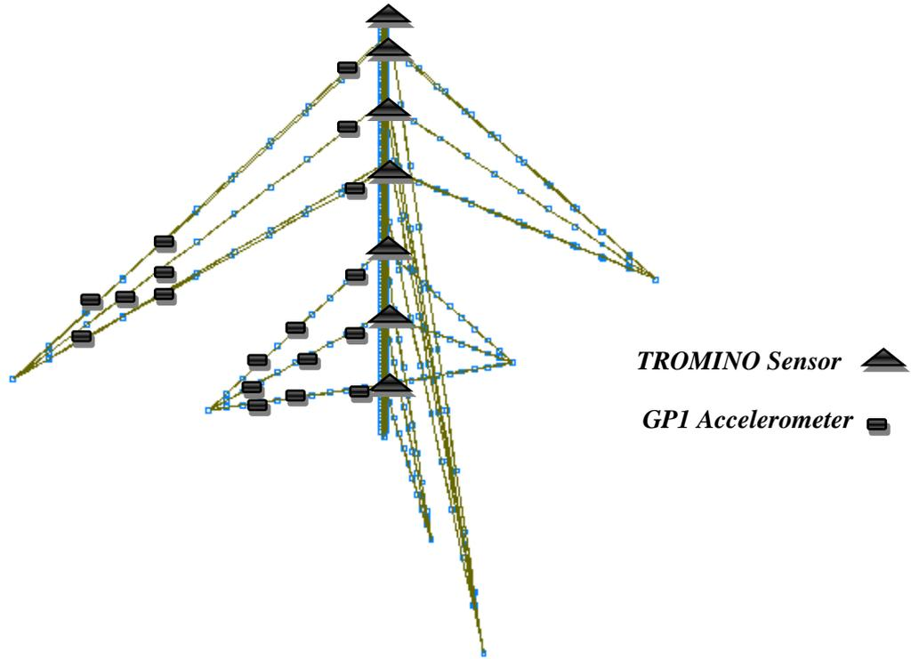
**Figure 2.2.** Location of the sensors on the tower
