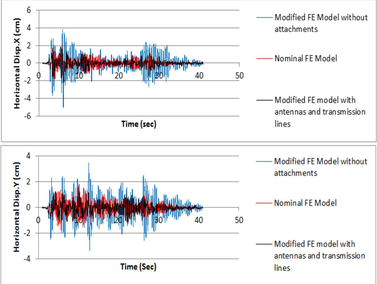
**Figure3.1.** Horizontal displacements of the mast at cable cluster elevation #6 (bottom cluster) along the X (along input) and Y (transverse to input)
