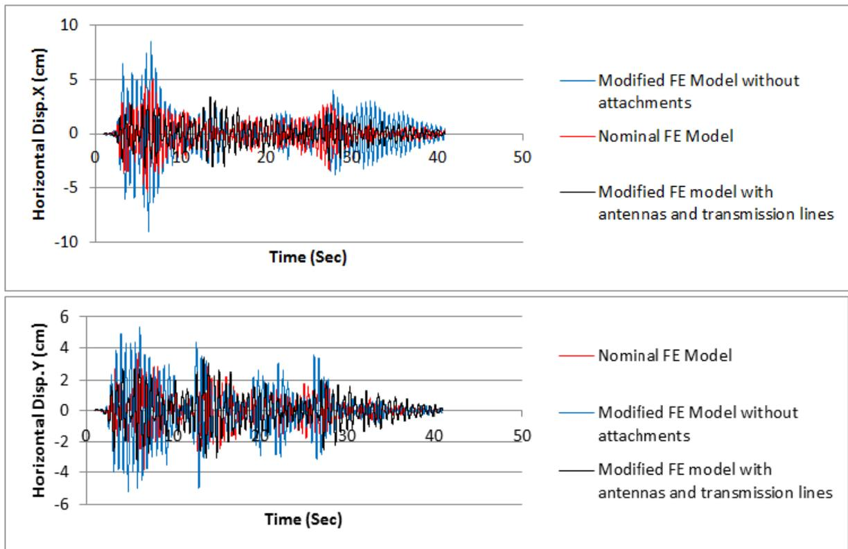
**Figure3.2.** Horizontal displacements of the mast at cable cluster elevation #1 (top cluster) along the X (along input) and Y (transverse to input)
