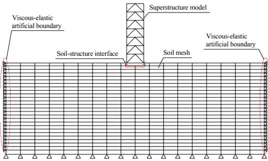
**Figure 3.1.** Soil-structure interaction model
