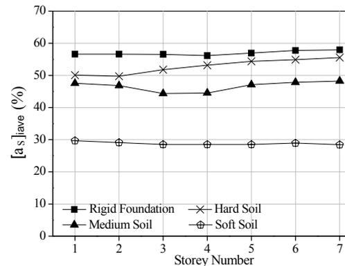
**Figure 5.2.** Storey drift reduction of each inter-storey
