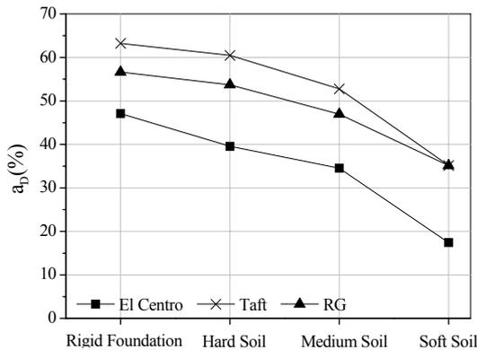
**Figure 5.1.** Relation curves of  $\alpha_D$  versus soil type
