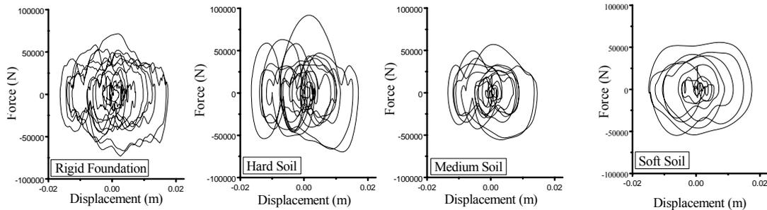
**Figure 5.3.** Hysteretic loops of the viscous damper installed in the bottom inter-storey
