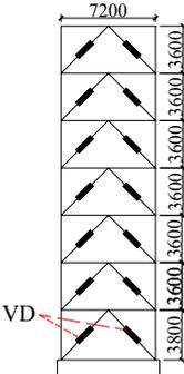
**Figure 2.1.** MRF retrofitted with VD
